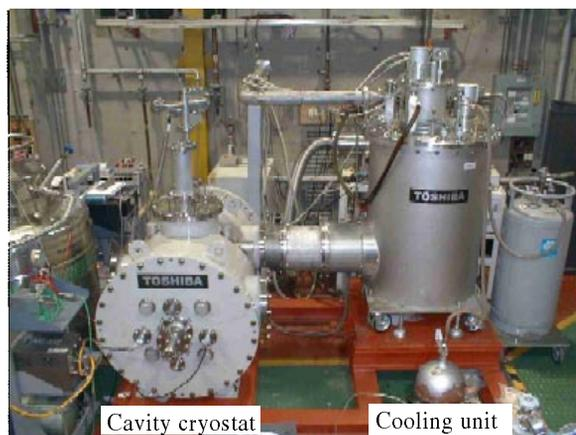
Figure 1: Cryomodule in a cooling test
