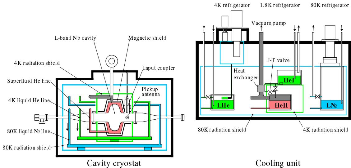
Figure 3: Schematic graph of the cryomodule
