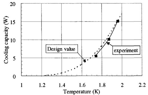
Figure 5: Cooling capacity of 1.8K line
