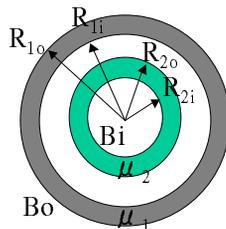
Figure 4: Formula of magnetic shielding for spherical shell[6]
