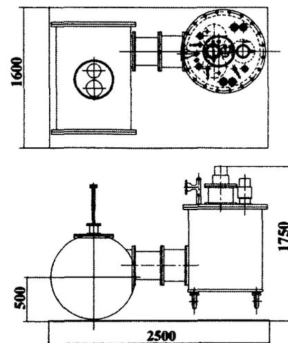
Figure 2: Dimensions(mm) of the cryomodule
