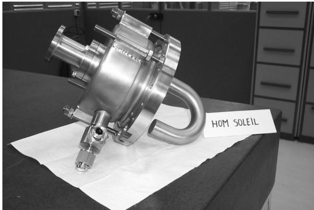
Figure 5: HOM coupler for dipole modes.
