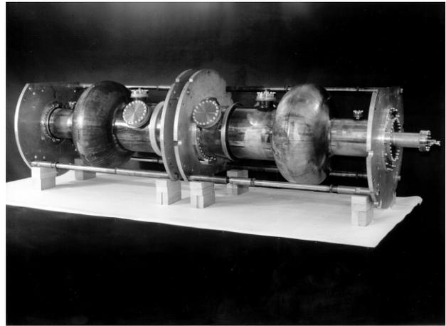
Figure 2: the two copper cavities after Nb deposition
