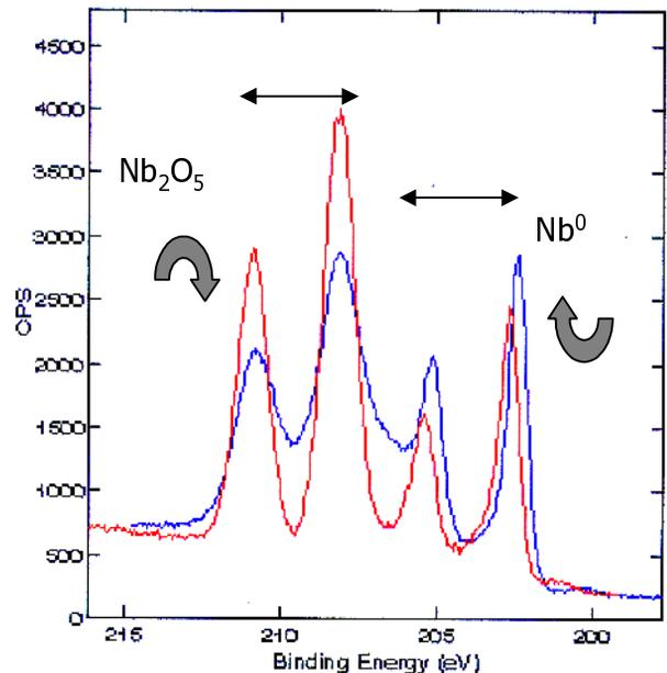
Figure 15 : Transformation of the niobium signal with baking : the Nb<sub>2</sub>O<sub>5</sub> signal decreases and gets wider will the Nb<sup>0</sup> signal increases slightly : the oxide layer has dissociated partly into suboxides and has got thinned.
