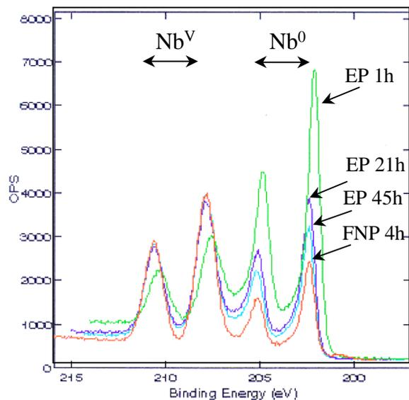
Figure 13 : Influence of air exposure on EP treated samples for the Nb signal.
