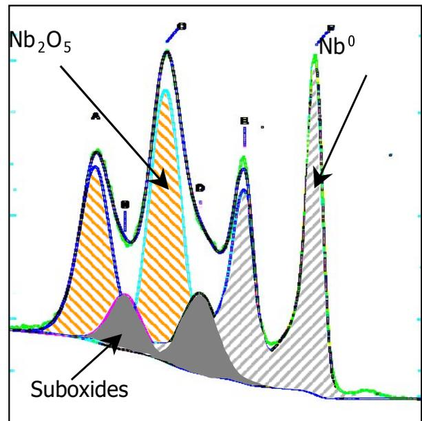
Figure 16 : Deconvolution of the niobium signal for the baked sample. The large signal of suboxides can probably be attributed to a mixture of Nb<sup>IV</sup> compounds.
