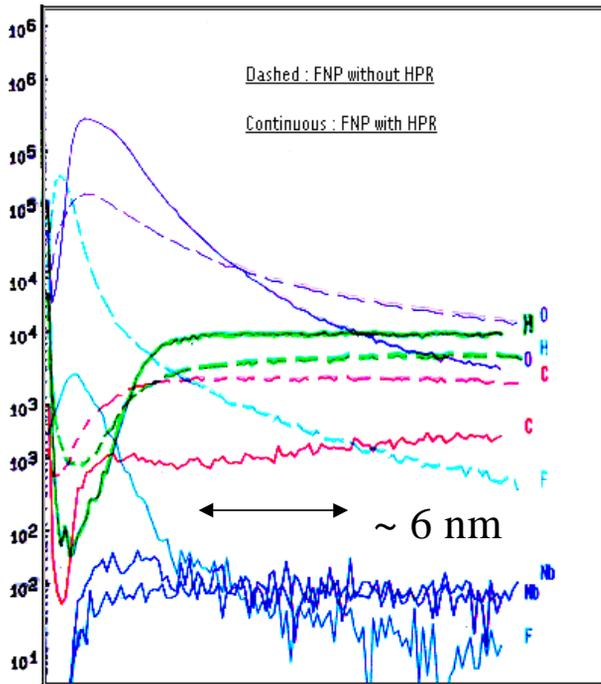
Figure 9 : SIMS profiling of FNP treated Nb samples, with or without high pressure rinsing. Depth scale deduced from ESCA results.
