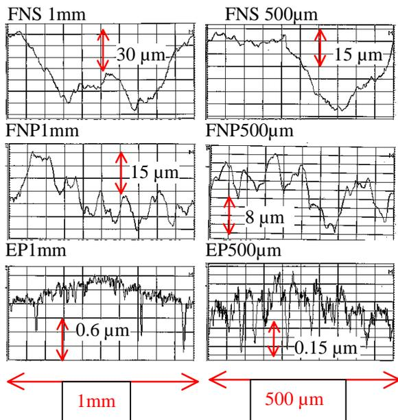
Figure 3 : profilometry at two different observing scale on Nb monocryстал. Results in term of Ra is showed in figure 5.
