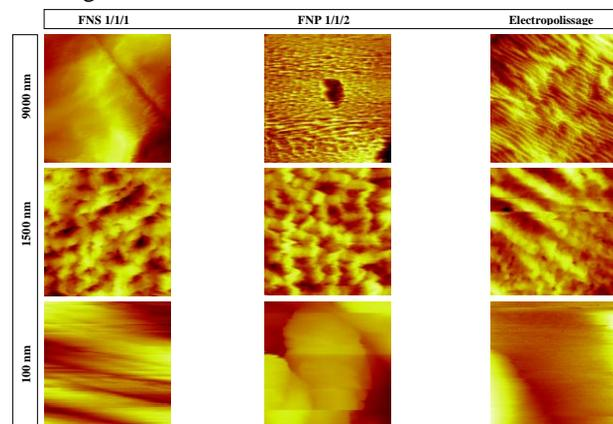
Figure 4 : Scanning Tunneling Microscope Images taken at three different observation scales, on Nb monocrystals treated with resp. FNS, FNP, and EP.
