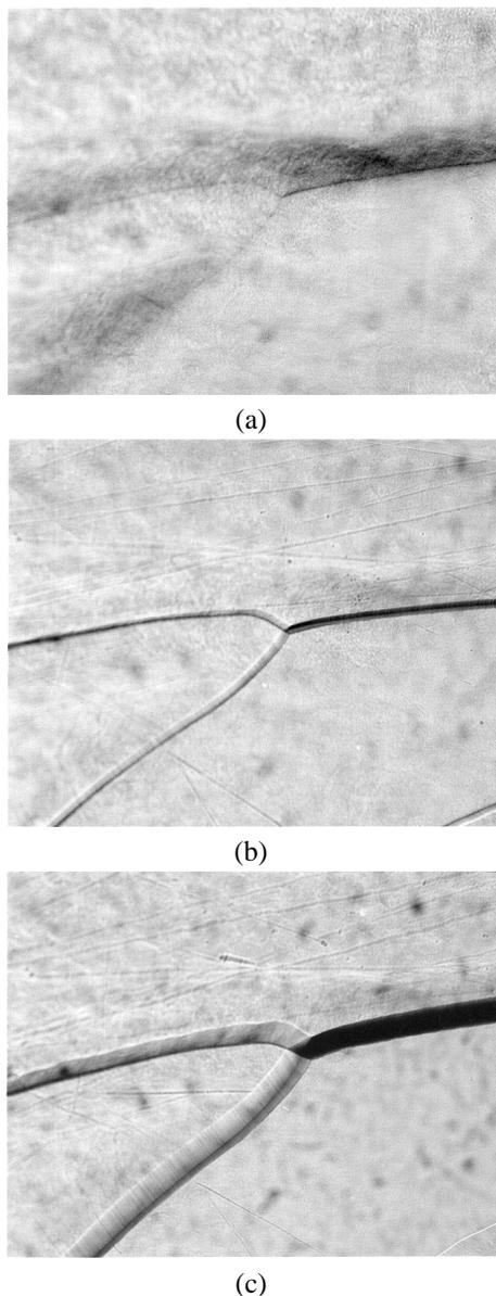
Figure 4: The weld surface of the sample S3C1-3-EQUATOR after EP followed by repeated BCP. After a surface removal of  $100\mu\text{m}$  by EP (a). After an extra removal of  $12\mu\text{m}$  (b);  $44\mu\text{m}$  (c) by BCP. The linear feature starting from the center to right is a going-down step if walking from the upper to the lower side in the picture.
