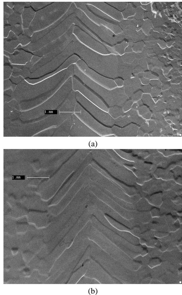
Figure 5: The RF surface of the weld and heat-affected region of the sample TWC-155E after a surface removal of  $117\mu\text{m}$  by BCP (a), and after an extra removal of  $90\mu\text{m}$  by EP. The length of scale bars in the photos is 1mm.
