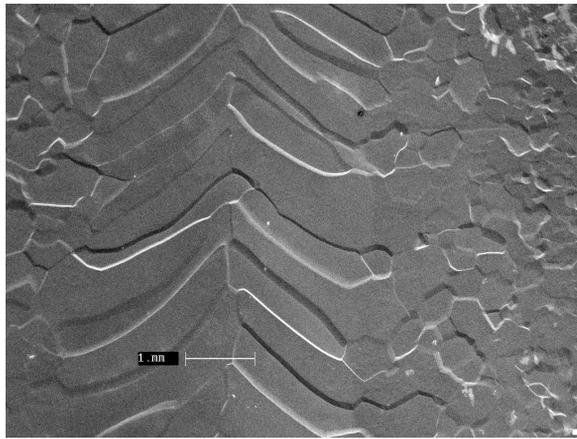
Figure 1: The SEM photo of the weld and heat-affected region of the sample TWC-155E after a surface removal of  $177\mu\text{m}$  by BCP. The length of the scale bar in the figure is 1mm.
