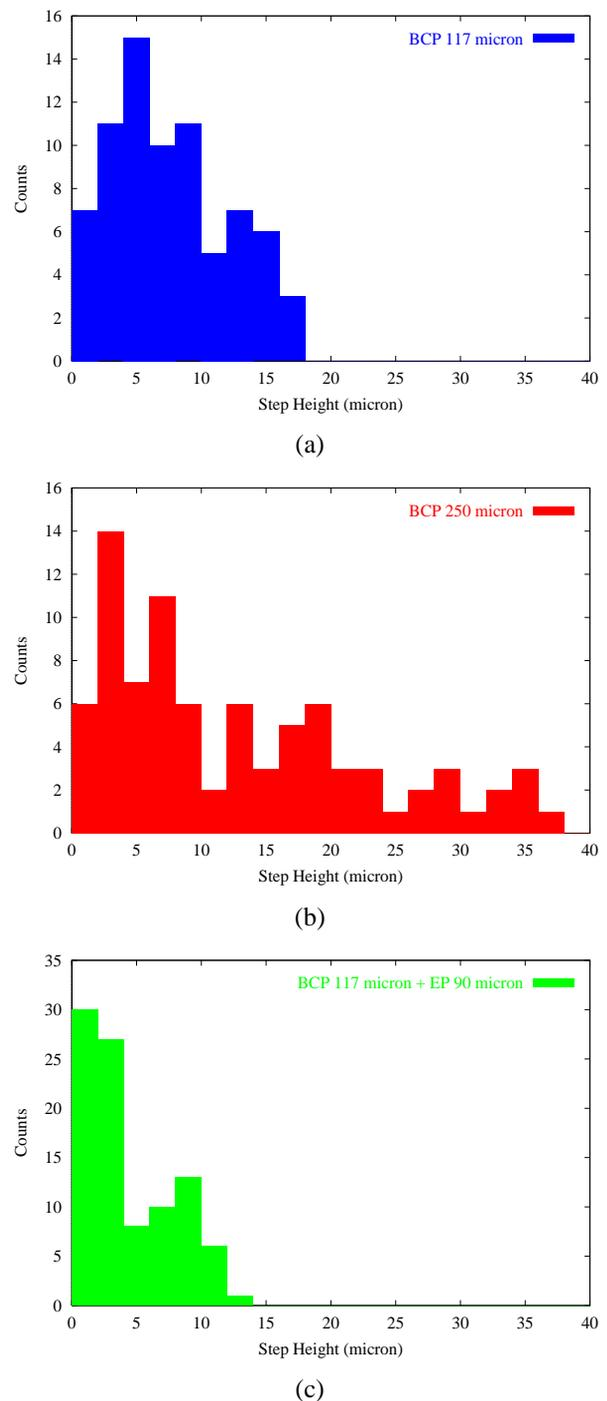
Figure 8: Histograms of step height in the weld region of the sample TWC-155E. After a surface removal of  $117\ \mu\text{m}$  (a). After a surface removal of  $117\ \mu\text{m}$  by BCP followed still by an extra  $133\ \mu\text{m}$  removal by BCP (b). After a surface removal of  $117\ \mu\text{m}$  by BCP followed by an extra  $90\ \mu\text{m}$  removal by EP (c).
