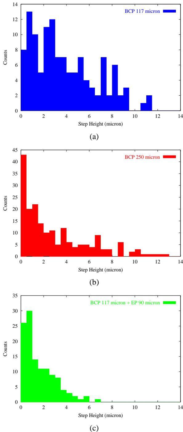
Figure 9: Histograms of step height in the non-affected region of the sample TWC-155E. After a surface removal of  $117\ \mu\text{m}$  by BCP (a);  $250\ \mu\text{m}$  (b). After a surface removal of  $117\ \mu\text{m}$  by BCP followed by an extra  $90\ \mu\text{m}$  removal by EP (c).
