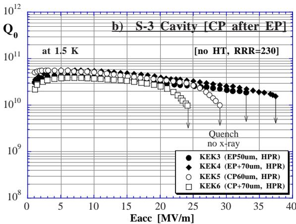
Figure 4-b): Cavity degradation due to CP after EP
