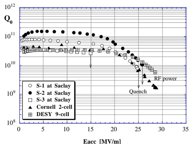
Figure 1: Test results at Saclay, Cornell and DESY
