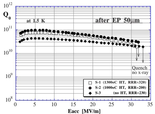
Figure 5: Three cavities after EP of 50 $\mu$ m
