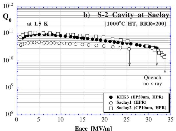
Figure 3-b): The S-2 cavity tested at Saclay
