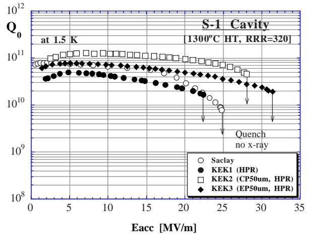
Figure 2: Test results in the S-1 cavity
