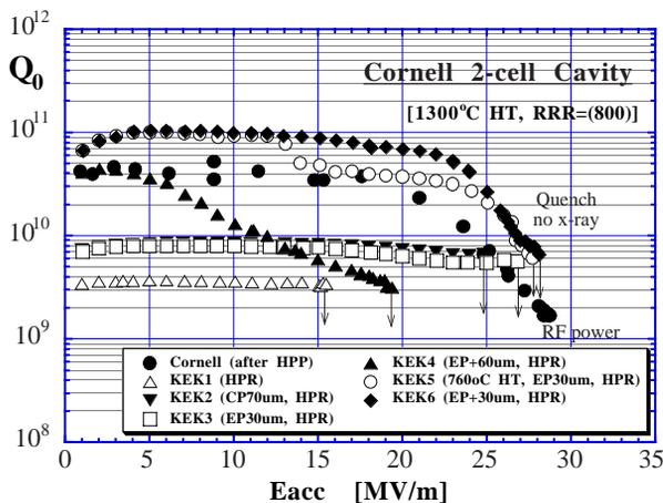
Figure 6: Test results in the Cornell two-cell cavity
