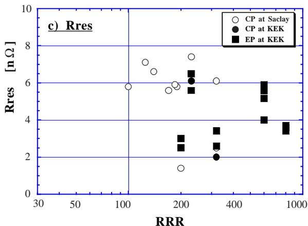
Figure 11-c): RRR dependence of the residual resistance
