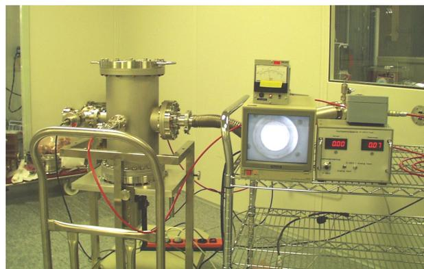
Figure 8: The apparatus for integral field emission measurement located inside the cleanroom.
