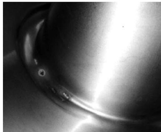
Figure 2: Photograph of cracks and exposed copper in electron-beam weld of resonator 304
