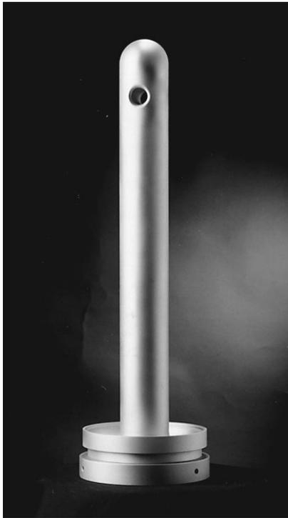
Figure 3: 150 MHz QWR for the booster LINAC at ANU
