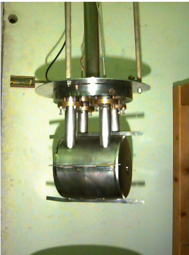
Figure 4, The PACO Cavity and the test Set-up.
