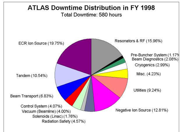
Figure 7. Distribution of causes of down-time at ATLAS in FY1998 (6050 hours total operating time).
