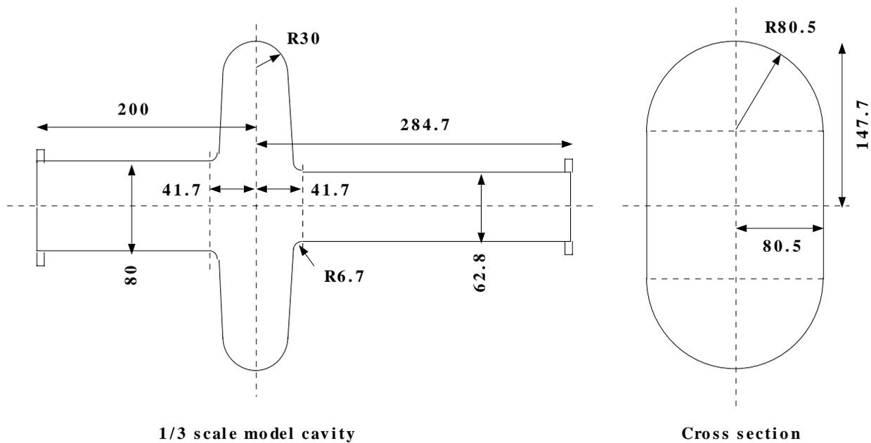
**Figure 1.** Dimension of 1/3 scale model cavity.
