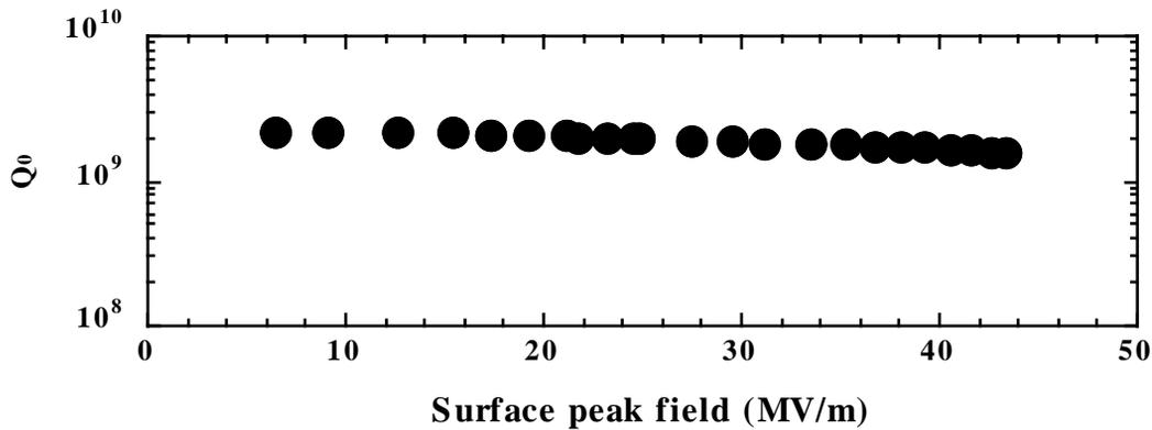
**Figure 2.**  $Q_0$  vs surface peak field.
