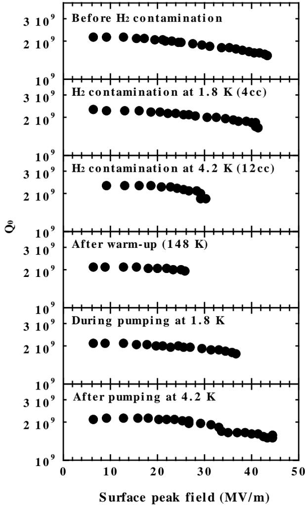
Figure 4. H<sub>2</sub> contamination test.
