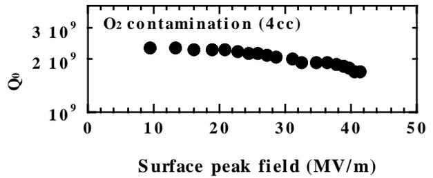
Figure 6. O<sub>2</sub> contamination test.
