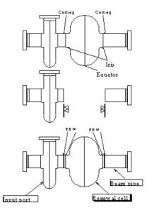
Fig.2 Removal processes of improper welded sections
