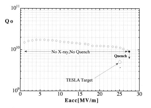
Fig.6  $Q_0$ -E<sub>acc</sub> plots in the cold test of the M-5 cavity
