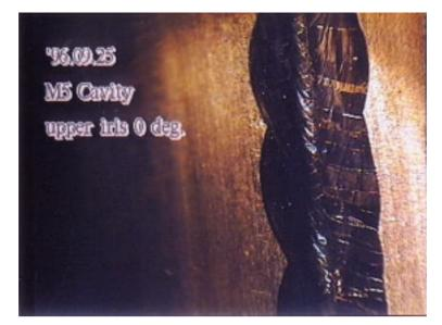
Fig.4 EBW seam in the M-5 Cavity
