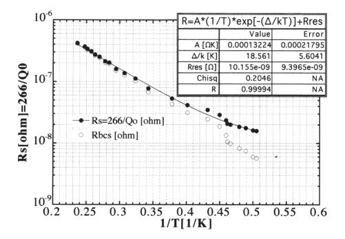
Fig.7 Temperature dependence of surface resistance the M-5 cavity
