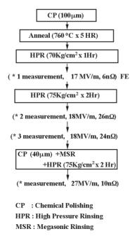
Fig.5 Surface treatment of the M-5 cavity (after repaired) 488 (2) Low-Temperature Performance Measurement Results
