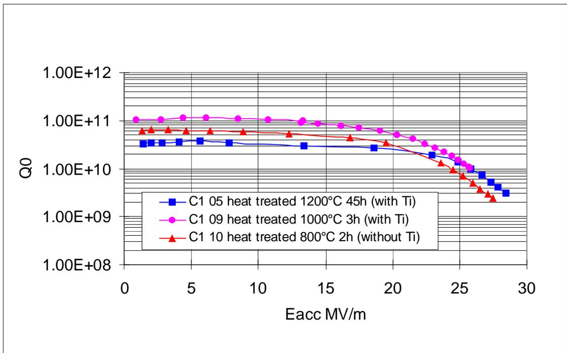
Fig. 1 : RF performances of cavities after different heat treatments
