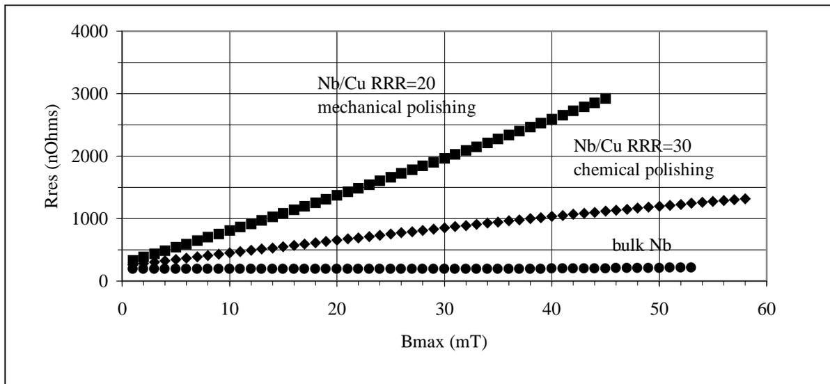
Fig.2 :Residual surface resistance of two different Nb coatings deposited on copper determined from RF measurements on TE012 mode at 5.7 GHz and T=1.7 K.
