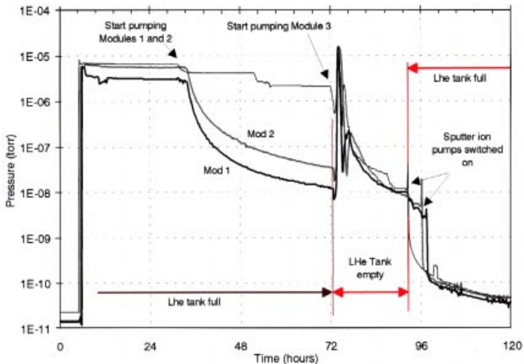
**Figure 3:** Evolution of the pressure in three different modules after He processing
