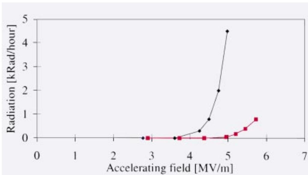
**Figure 1.** Effect of *in situ* pulse processing of different modules in LEP. The diamonds represent the radiation before processing; the squares show the radiation after processing.
