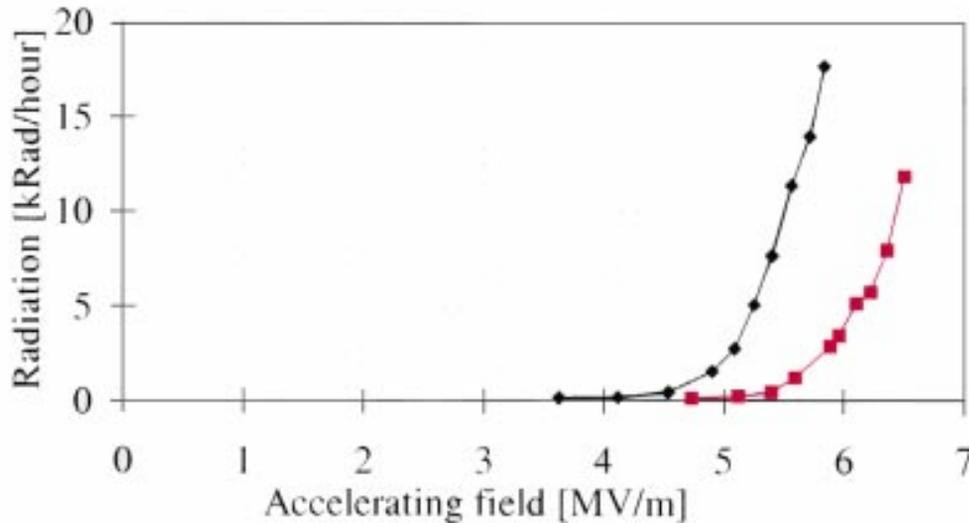
**Figure 2.** Effect of *in situ* He- processing of a module in LEP. The diamonds represent the radiation from the modules before processing; the squares show the radiation after processing. After only a few hours of processing the radiation emitted by the modules was significantly reduced.
