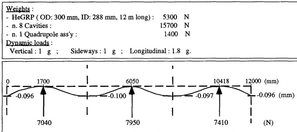
Fig. 6- Loads and HeGRP computed deflection under load
