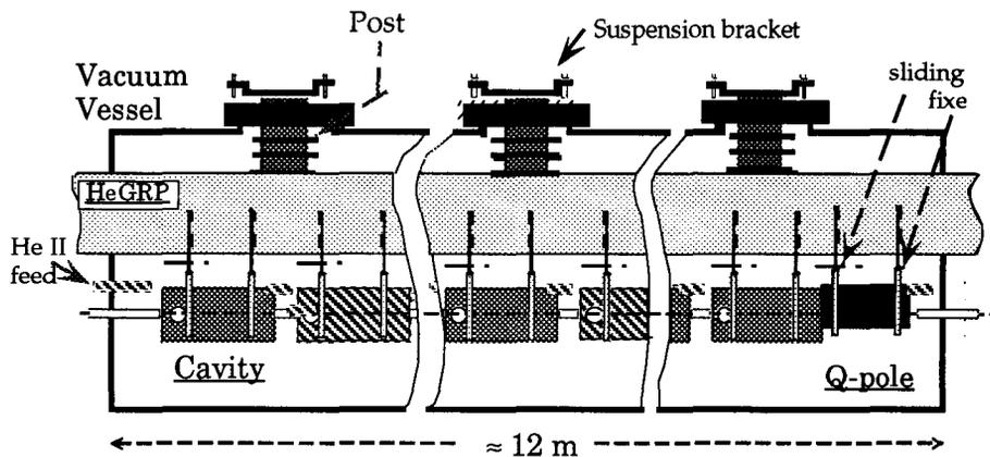
Fig. 2. - Schematic view of the cryostat
