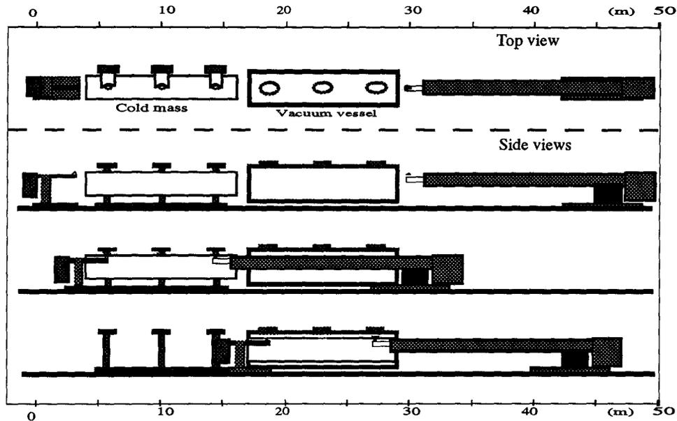
Fig. 9. - Schematic view of the AM insertion into the cryostat sequence.
