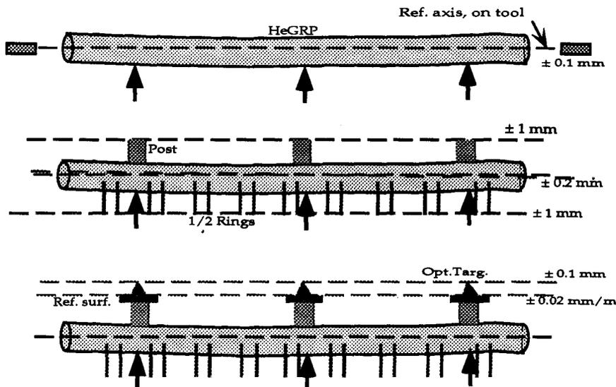
Fig.7. - Sketch of the AM suspension system first assembly phases
