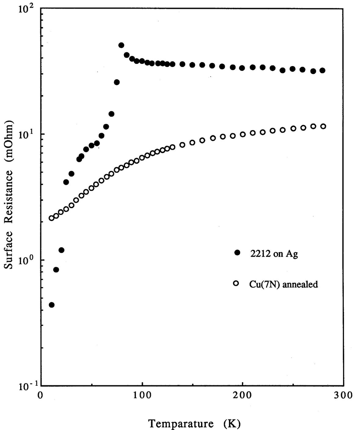
Fig.3 Surface resistance vs. temperature for BSCCO on Ag and Cu(7N) around 2.2GHz
