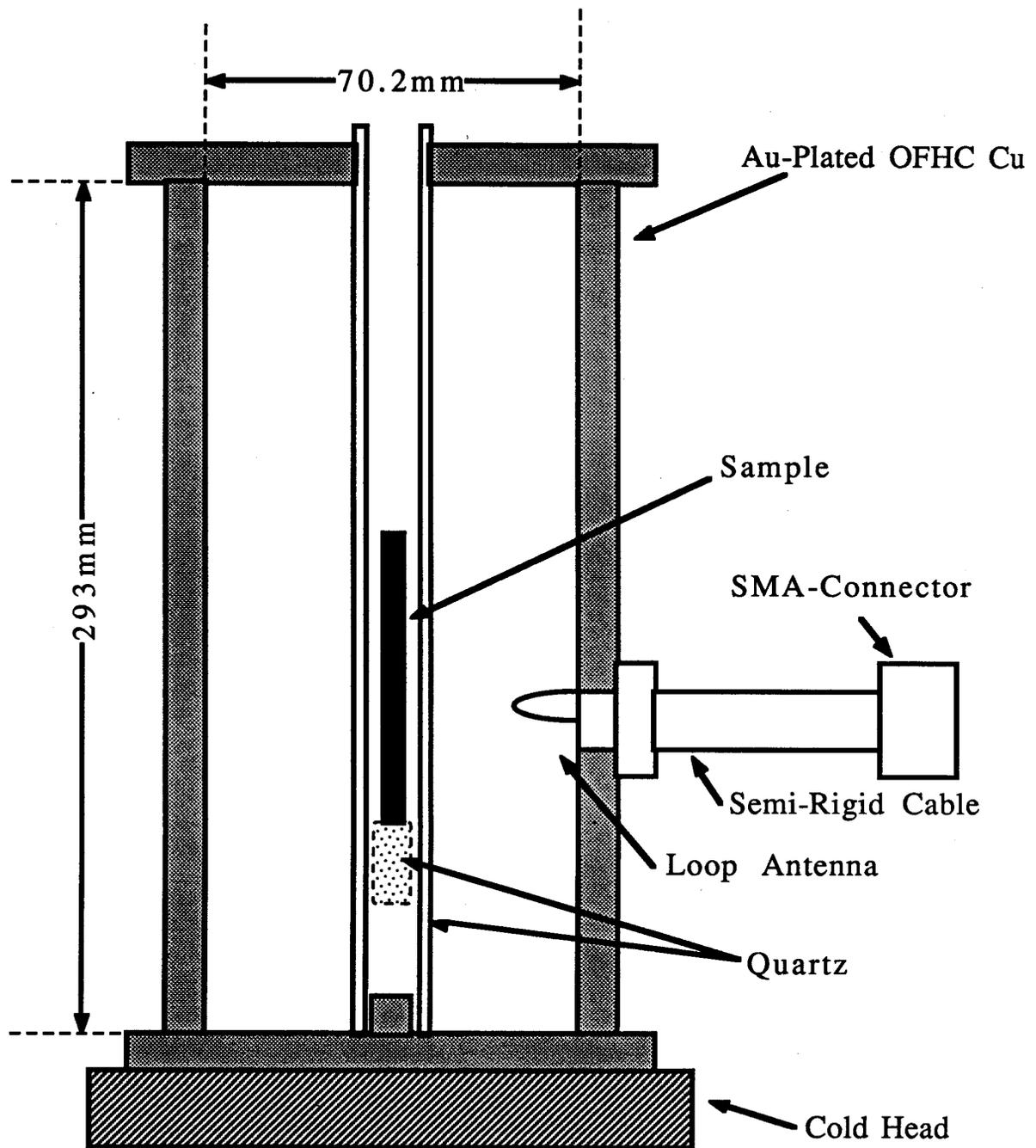
Fig.2 A half-wave coaxial cavity resonator
