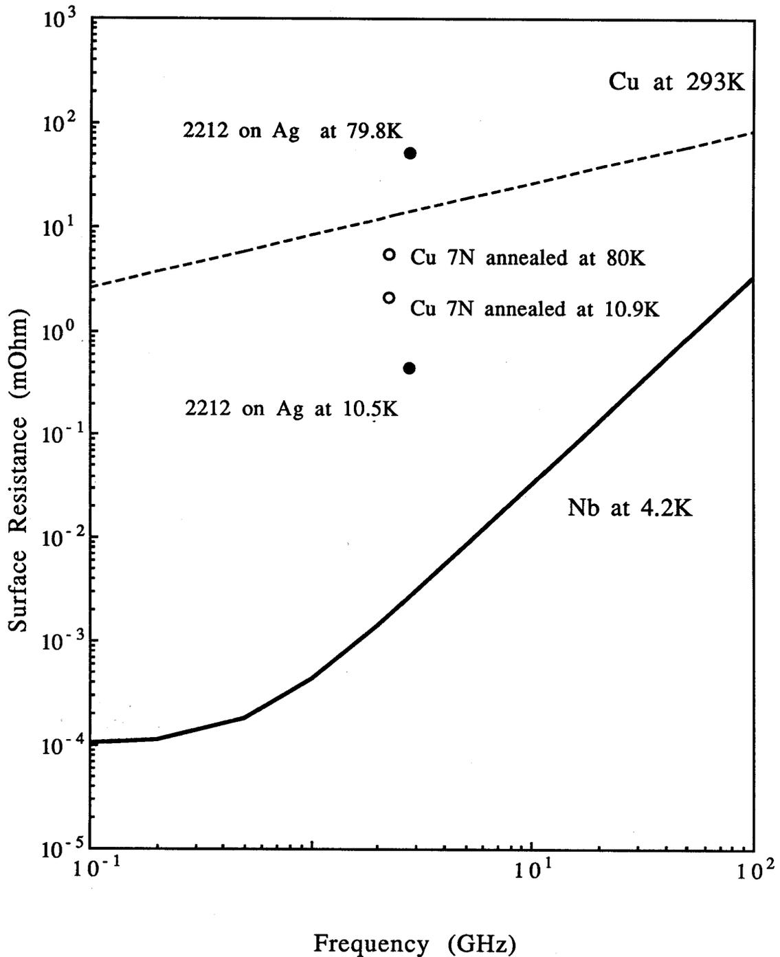
Fig.4 Surface resistance vs. frequency for BSCCO on Ag and Cu(7N) around 10 and 80K
