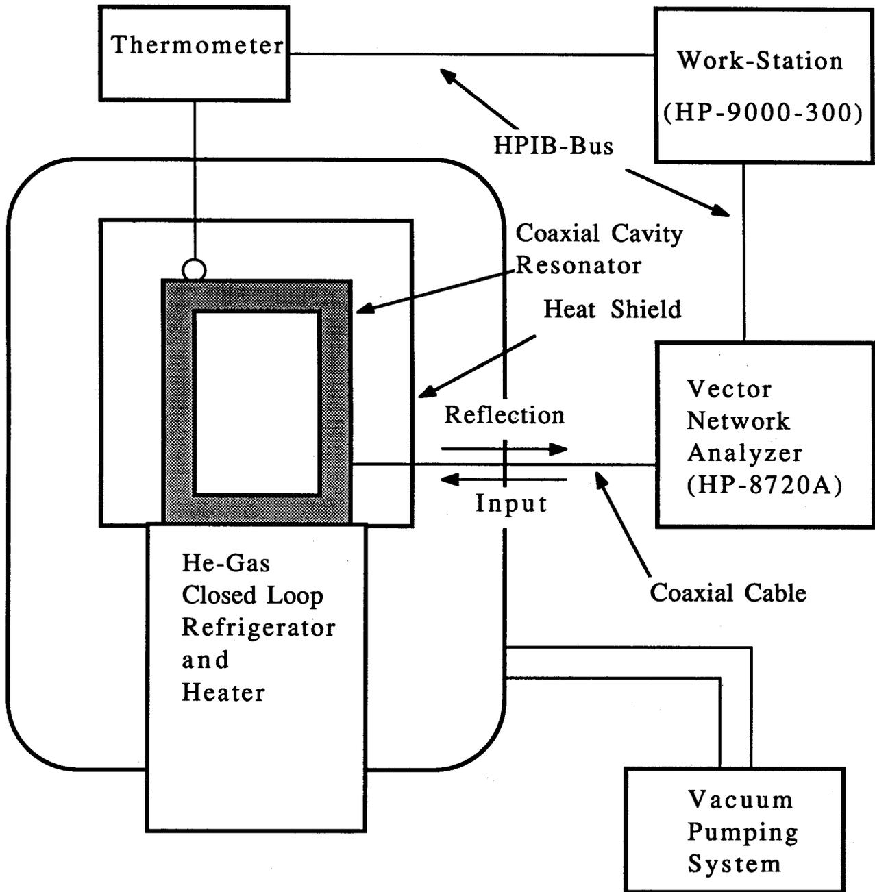
Fig.1 Schematic diagram of the experimental setup
