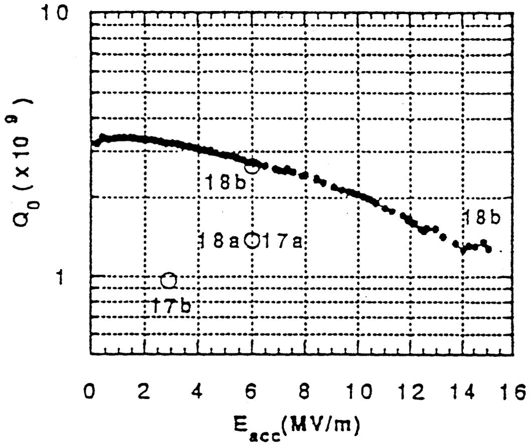
Fig. 6: Best result obtained with an electropolished 500 MHz-cavity at KEK
