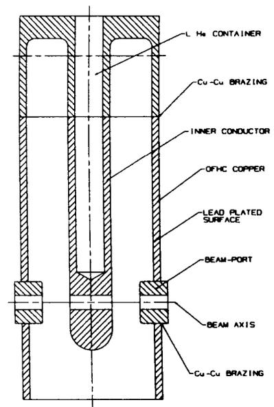
Fig. 2. 160 MHz,  $\beta_o = 0.11$  copper resonator.
