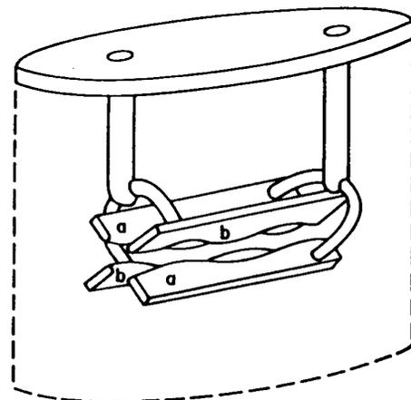
Fig. 6. Schematic drawing of a  $2\beta\lambda$  RFQ resonator.
