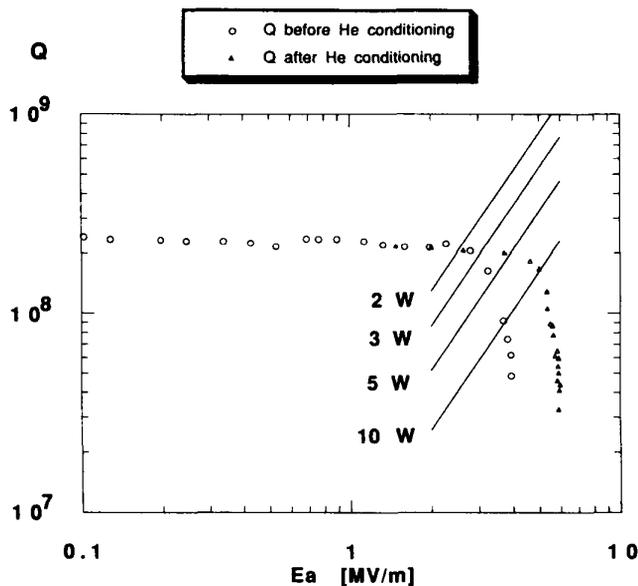
Fig. 5. Medium  $\beta$  niobium resonator performance at 4.2 K.
