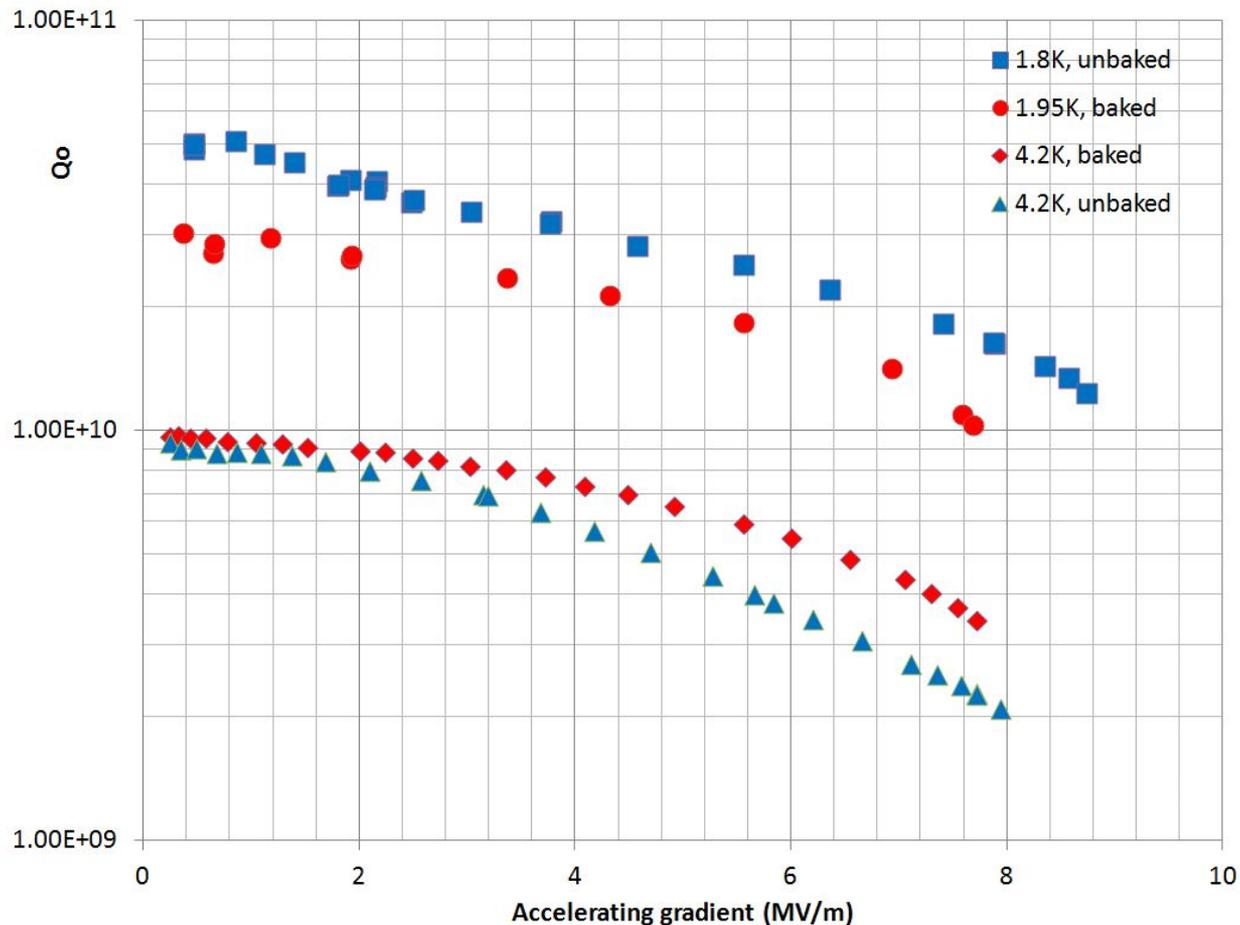
At low frequency, 120°C baking is justified if operated at 4.2K.
