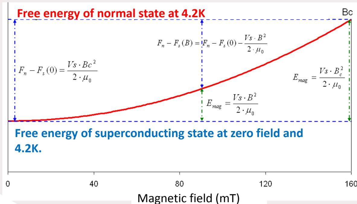
$$\Delta(T, B) = \Delta(T, B = 0) \cdot \left(1 - \left(\frac{B}{Bc(T)}\right)^2\right) \quad Bc(T) = Bc(0) \cdot \left(1 - \left(\frac{T}{Tc}\right)^2\right)$$
