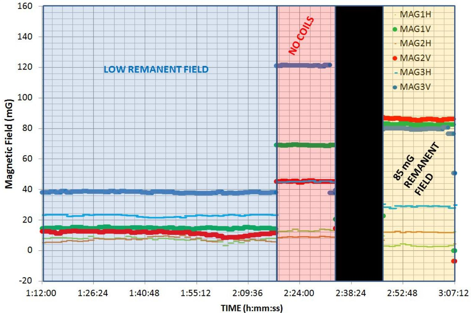
Magnetic configurations to study magnetic sensitivity of cavity
