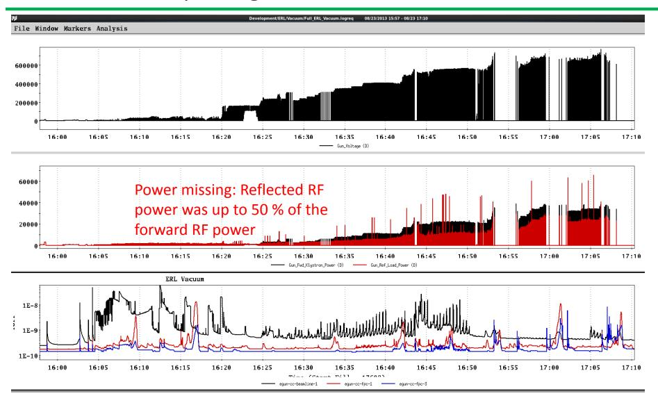
After conditioning for 7 days and average 10 hours per day, the gun reached 1.85 MV with 18% of duty factor.
