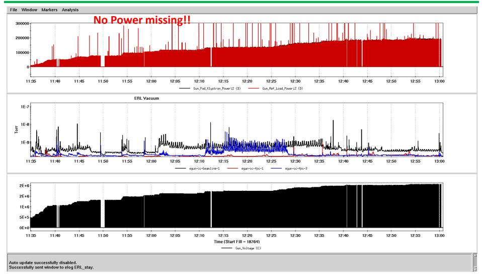
➤ Within the first 1.5 hours, the cavity voltage goes up to 2 MV in pulse mode without multipacting.
