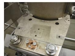
Cavity mount provides stress free thermal contraction with significant anti-rocking stiffness
