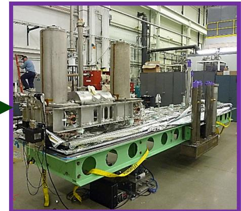
Coldmass Installed to Baseplate
