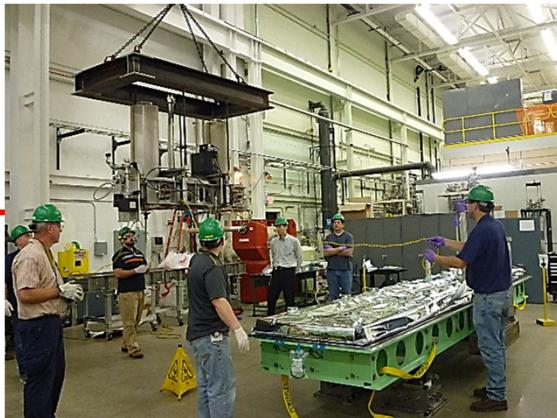
Installation of Lower Magnetic Shield and Tuner to Coldmass
