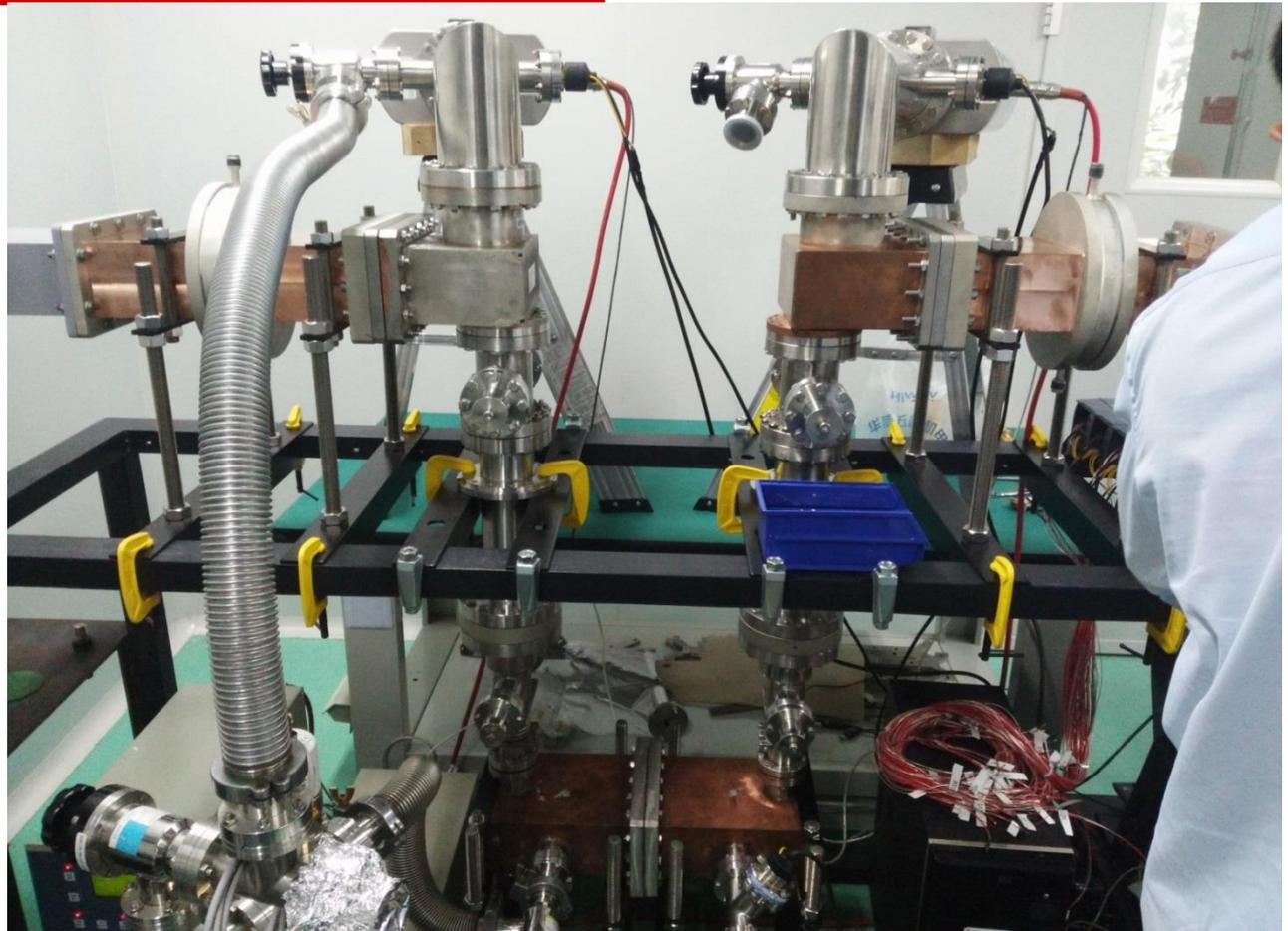
**Both couplers can transfer 10kW RF power with 10Hz and a duty factor of 30%**
