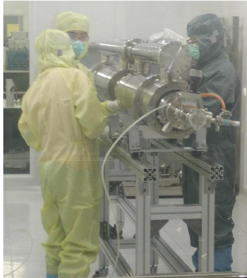
**Assembly of the two 9-cell cavities**
