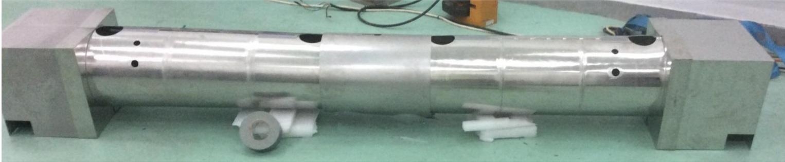
Magnetic shield for  $2 \times 9$ -cell cavity: low temperature permalloy
