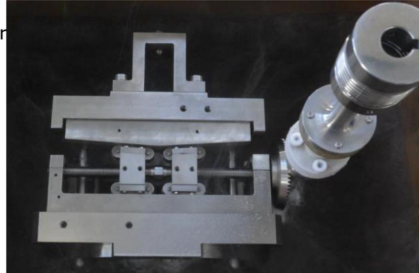
**Tuning system includes one step motor and two piezos**
