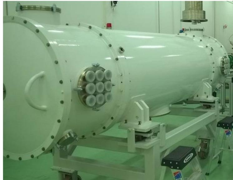
Vacuum vessel of the cryomodule
