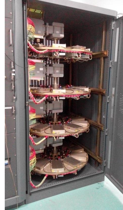
Three 10kW 1.3GHz solid-state RF power amplifiers.
