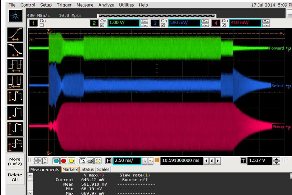
RF signals for beam loading experiment
