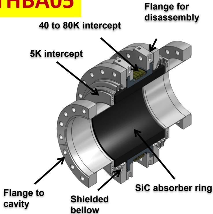
Beamline HOM absorbers strongly damp dipole HOMs to under  $Q \sim 10^4$
