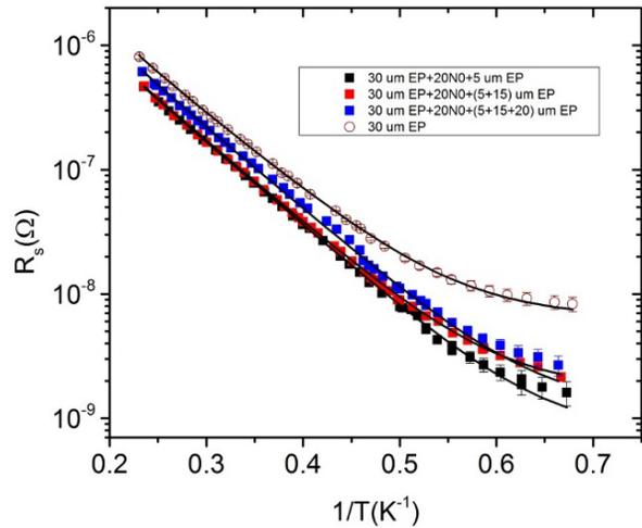
Figure 4: Surface resistance data from TD-5 taken at  $\sim 8$  mT. Data and fit of  $R_s$  vs  $1/T$  using the BCS theory as described in text to extract the superconducting parameters. Fitting is using the Halbritter code.
