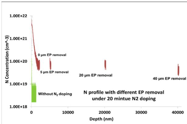
Figure 6: Nitrogen content at the surface of witness samples treated in the same furnace run as RDT-13 and TD-5. EP performed with the same parameters, but in different setup.
