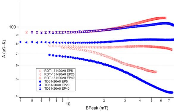
Figure 2: Temperature dependent "A" fitting parameter vs. field for all three dopings for both RDT-13 and TD-5, data taken before 120 K soak, data admin limited to 75 mT or first quench.
