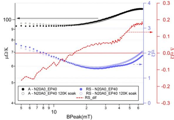
Figure 5:  $RS$ ,  $A$ , and differences in  $RS$  before and after 120 K soak for 5 hour (10 hours above 90 K) on RDT-13 N20A0\_EP40.
