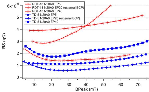
Figure 3: Temperature independent "RS" fitting parameter vs. field for all three dopings for both RDT-13 and TD-5, data taken before 120 K soak, data admin limited to 75 mT or first quench.
