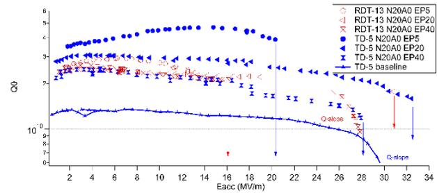
Figure 1:  $Q_0$  vs.  $E_{acc}$  for all tests before thermal cycles, including TD-5’s non-doped baseline test. Down arrows represent quench fields.
