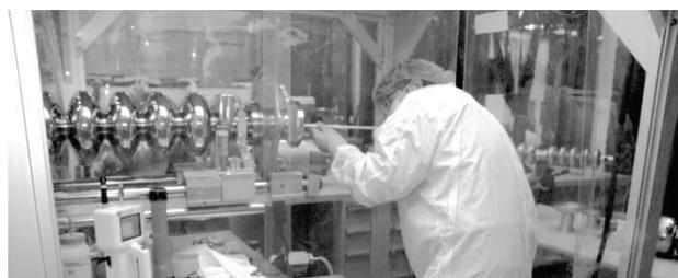
Figure 1: Particulate collection from cavity inner surface.
