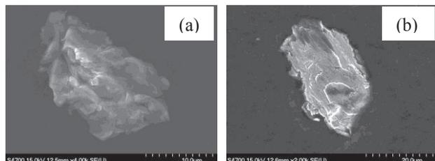
Figure 3: (a) A “clay” particulate collected from the beam tube of cavity IA080; (b) A stainless-steel particulate collected from the beam tube of cavity IA351.
