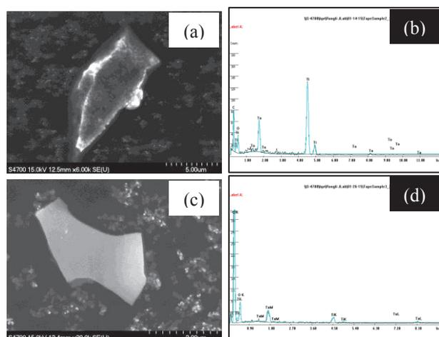
Figure 2: Titanium/tantalum particulates. (a) This 10  $\mu\text{m}$  sized particulate is collected from niobium beam tube surface of cavity IA355; (b) EDX spectrum of particulate shown in (a). (c) This 4 $\mu\text{m}$ -sized particulate is collected from the first iris of cavity IA351; (d) EDX spectrum of particulate shown in (c).
