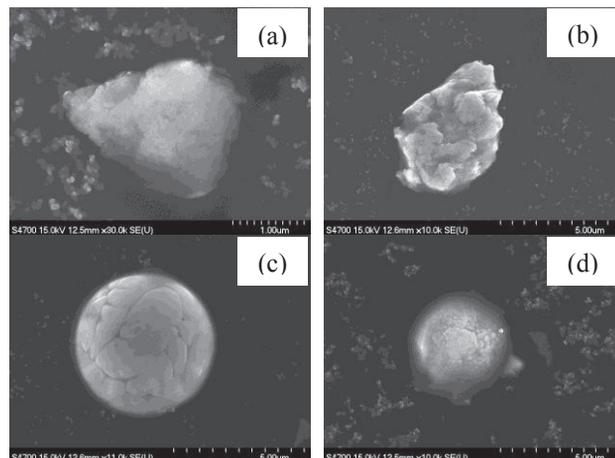
Figure 4: (a) A 2 μm sized copper particulate collected from the beam tube/first iris region of cavity IA351; (b) A niobium particulate collected from the first iris of cavity IA080; (c) A spherical iron particulate collected from the beam tube of cavity IA080; (d) A near spherical particulate with granule sub-structures, consisting of multiple elements including iron, chromium, nickel and sulfur, collected from the second iris of cavity IA290.
