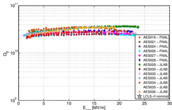
Figure 4: 2K  $Q_0$  vs  $E_{acc}$  performance of dressed N-doped cavities in vertical test.  $Q_0$  values are corrected for cavity flange losses during performance testing, which will not be present in LCLS-II cryomodule installation.
