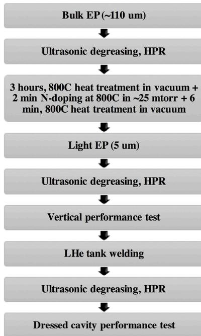
Figure 2: Baseline cavity preparation process for LCLS-II production cavities.
