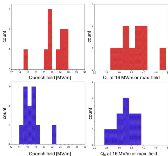
Figure 1: Top: 2K nine-cell cavity performance values using the "2N6A" nitrogen doping recipe. Average quench field: 22.2 MV/m. Average  $Q_0$ :  $3.6 \times 10^{10}$ . Bottom: 2K nine-cell cavity performance values using the "20N30A" nitrogen doping recipe. Average quench field: 16.3 MV/m. Average  $Q_0$ :  $3.2 \times 10^{10}$ .
