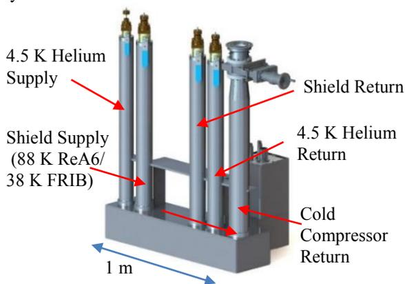
Figure 6: Cryomodule cryogenic bayonet box. The bayonet box connects to the distribution line by u-tube bayonets. The box is shown as it would supply for FRIB.
