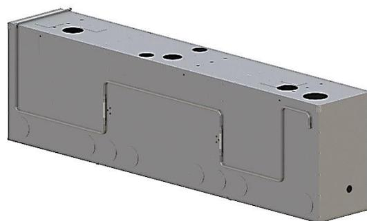
Figure 11; Value engineering was applied to the thermal shield for the FRIB Beta=0.085 cryomodule design to utilize a panelized configuration.
