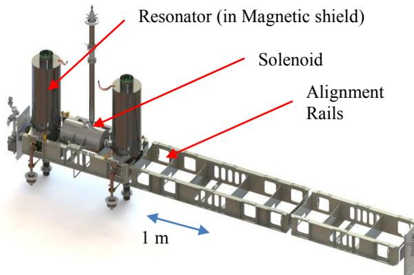
Figure 4: Cryomodule cold mass. Alignment rails support superconducting resonators and solenoid.
