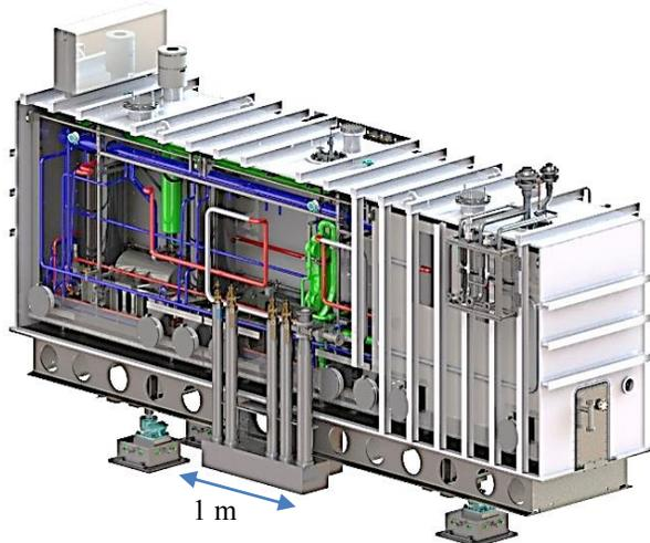
Figure 2: ReA6 modular bottom-up cryomodule design. This cryomodule incorporates 2  $\beta=0.085$  QWRs and 1 solenoid.
