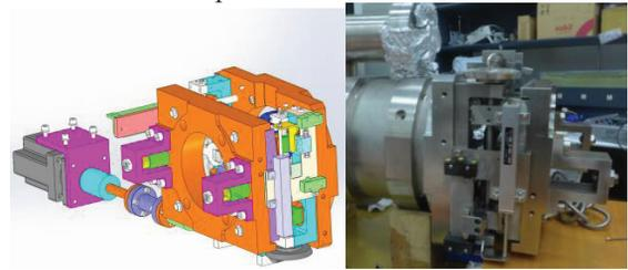
Figure 5: slow and fast tuner for a 9-cell cavity.
