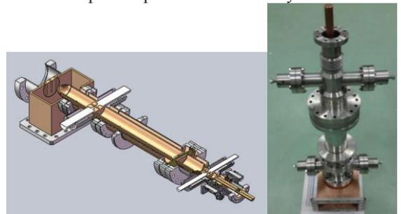
Figure 6: input coupler for the 9-cell cavity.
