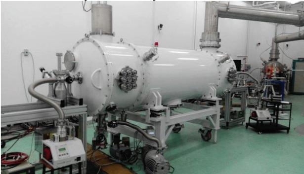
Figure 7: Layout of the 9-cell cryomodule and the DC-SRF photoinjector.
