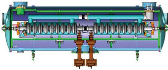
Figure 3: The sectional view of the 2 × 9-cell superconducting cavity cryomodule.
