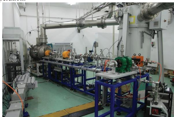
Figure 2: Beam experiment layout of the DC-SRF photoinjector.
