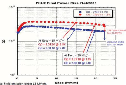
Note: Field emission onset 15 MV/m, Maximum X-ray dose rate < 100 mR/hr. No more mode mixing observed during final power rise.
