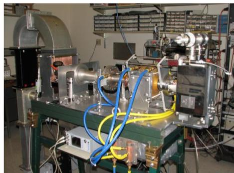
Figure 9: High Power Input Coupler test stand
