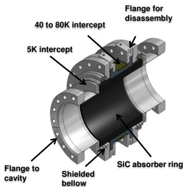
Figure 6: cross section view of HOM
