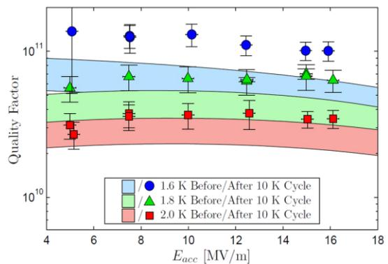
Figure 4: Q(E) before/after thermal cycle
