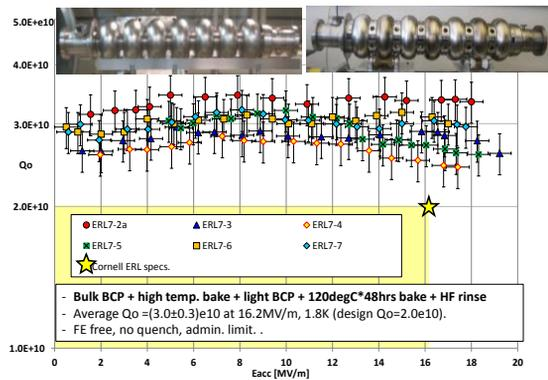
Figure 2: VT results of ERL 7-cells at 1.8K
