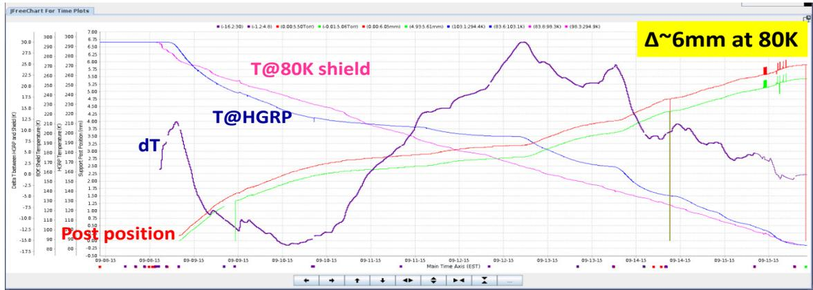
Figure 16: Position of sliding posts during cooldown
