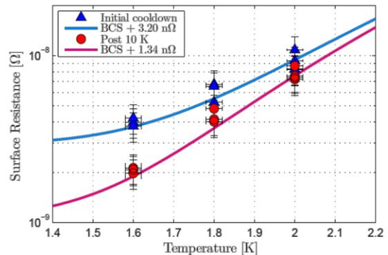
Figure 5: Rs before/after thermal cycle
