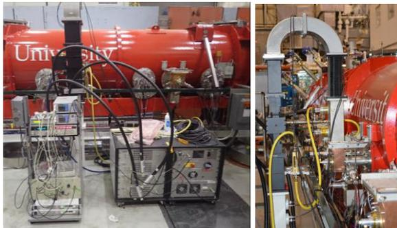
Figure 17: MLC cavity RF test set-up
