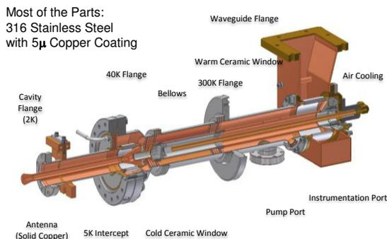
Figure 8: High Power Input Coupler for MLC
