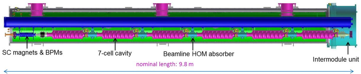
Figure 1: Cornell ERL Main Linac Prototype Cryomodule
