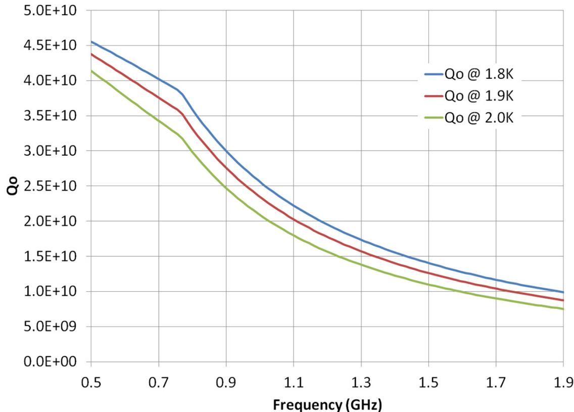
**Q<sub>0</sub> as a function of frequency and temperature at 16 MV/m. All frequencies scaled from CEBAF C100 upgrade cavity.**
