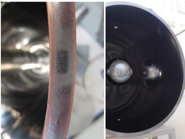
Figure 4: RF contact surfaces after rinsing: adhesion improved using a longer sputtering cathode.
