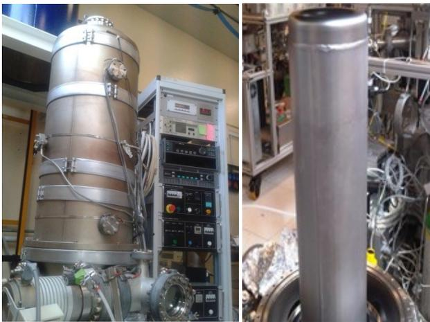
Figure 5 HIE-ISOLDE sputtering system at INFN-LNL.
