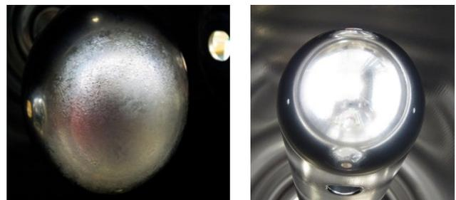
Figure 3: Surface of the inner conductor tip before and after removing the central electrode.
