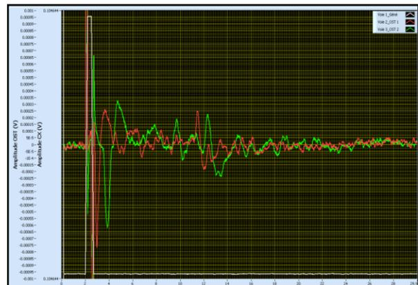
Fig. 13: Response of OST #1 (red) and OST #2 (green), at  $T_{bath} = 2.1$  K to a pulsed heat flux  $q_p = 753$  W/cm<sup>2</sup>, with  $\tau_p = 100 \mu s$  for  $V_p = 150$  V-Test cell#3: Flat SMD heater area = 5.1 mm<sup>2</sup>.
