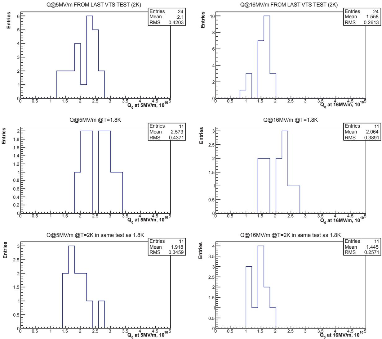
Figure 4:  $Q_0$  at 5MV/m and 16MV/m for Fermilab cavities at 2K. Left:  $Q_0$  at 5MV/m. Right:  $Q_0$  at 16MV/m. Top: 2K measurements. Middle: 1.8K measurements. Bottom: 2K measurements for the sub-sample that corresponds to 2K measurements.
