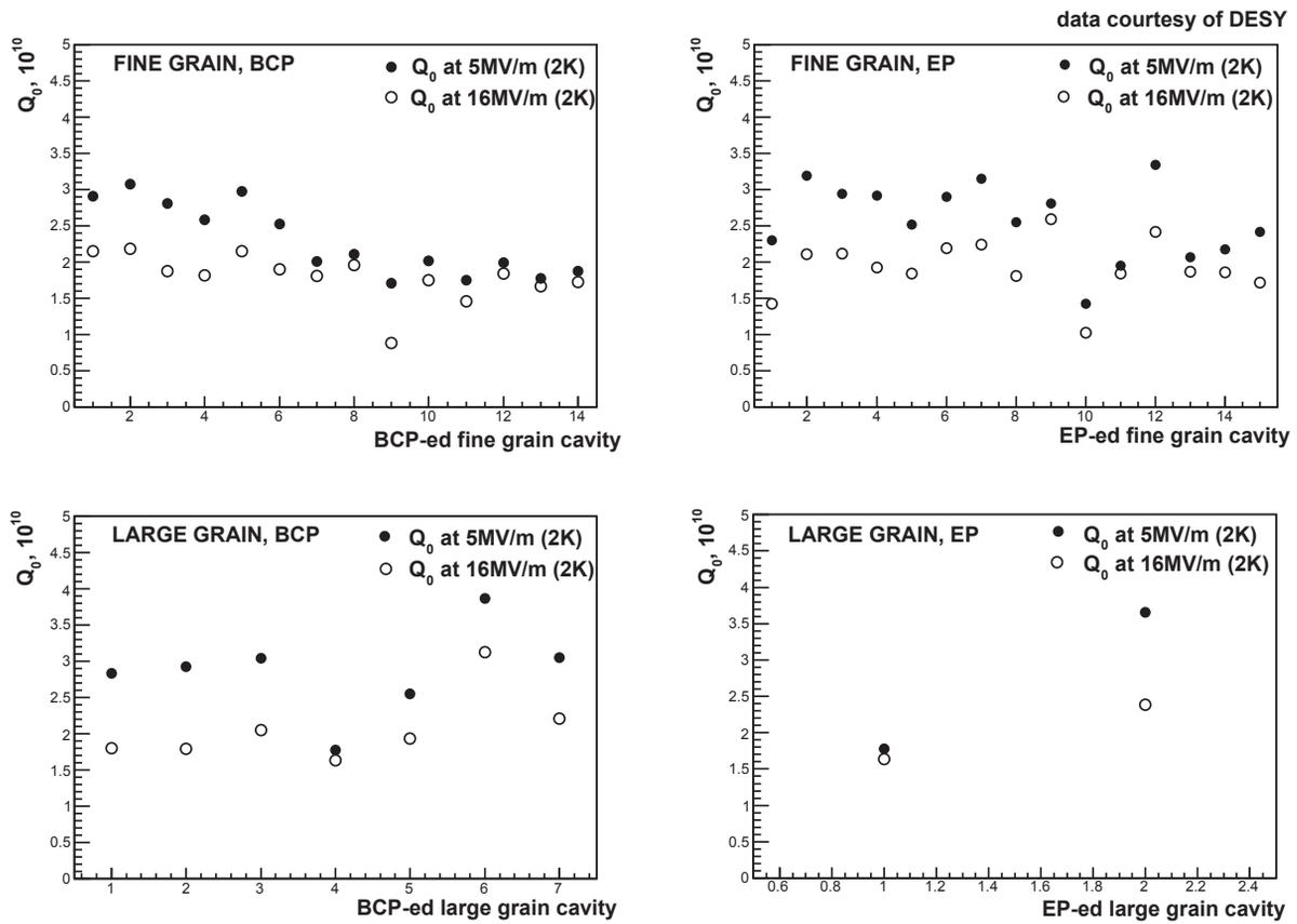
Figure 2:  $Q_0$  at 5 MV/m and 16 MV/m for large grain DESY cavities
