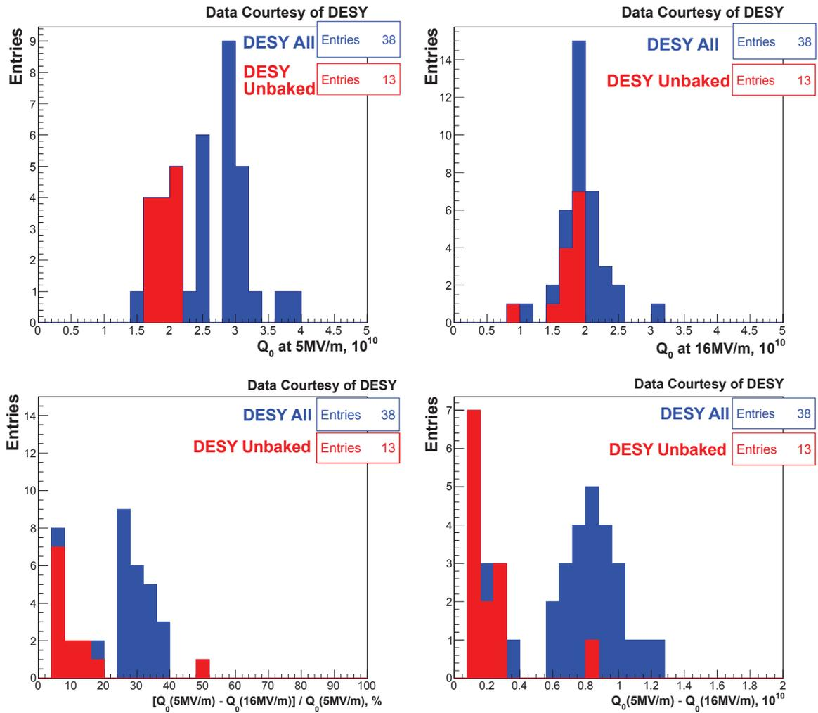
Figure 3: Comparison between all DESY cavities (blue) and low temperature unbaked DESY cavities (red). Top left:  $Q_0$  at 5MV/m. Top right:  $Q_0$  at 16MV/m. Bottom left: relative MFQS. Bottom right: and absolute MFQS
