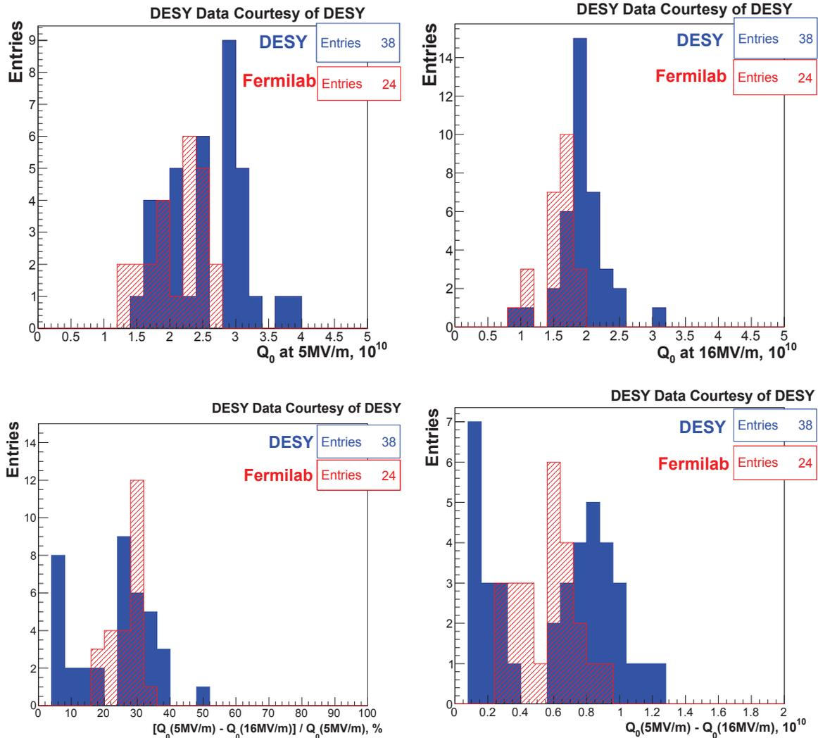
Figure 1: Comparison between DESY (solid blue) and Fermilab (hatched red) cavities. Top left:  $Q_0$  at 5 MV/m. Top right:  $Q_0$  at 16 MV/m. Bottom left: relative MFQS. Bottom right: and absolute MFQS
