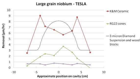
Figure 1: CBP removal rate for large grain niobium as a function of cavity position. The physical profile of the cavity is shown in thin black.
