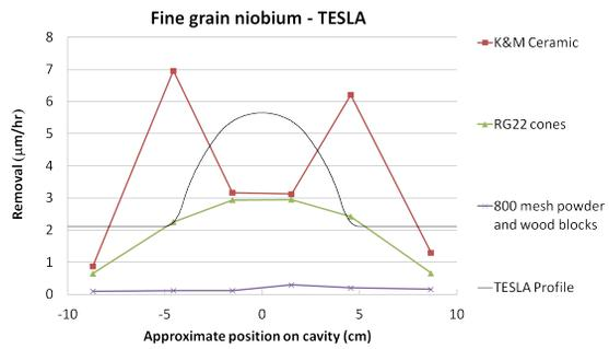
Figure 3: CBP removal for TESLA fine grain niobium. The physical profile of the cavity is shown in thin black line.
