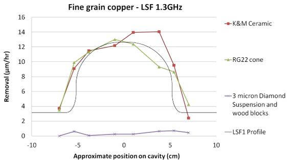
Figure 2: CBP removal rate for low surface field 1.3 GHz, 1/2 hardness copper as a function of cavity position. The physical profile of the cavity is shown in thin black.
