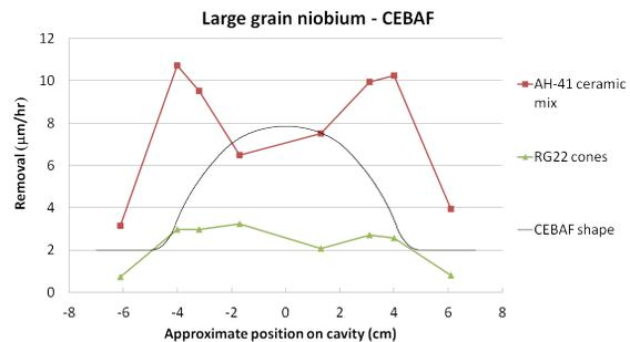
Figure 4: CBP removal rates for large grain niobium CEBAF shape. The physical profile of the cavity is shown in thin black line.
