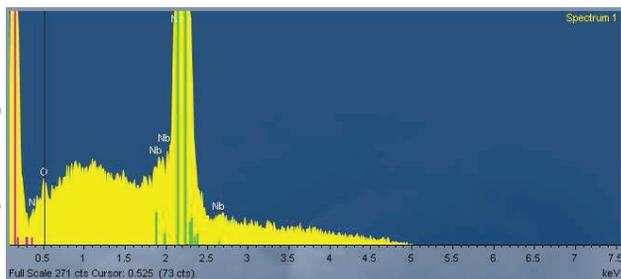
Figure 5: EDX spectrum of sample #7 showing unpopulated Nitrogen lines.
