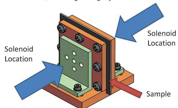
Figure 1: Sketch of the inductive T<sub>c</sub> measurement apparatus. The sample under test is placed between two coils decoupling their magnetic field if the sample is in the superconducting Meisner state.
