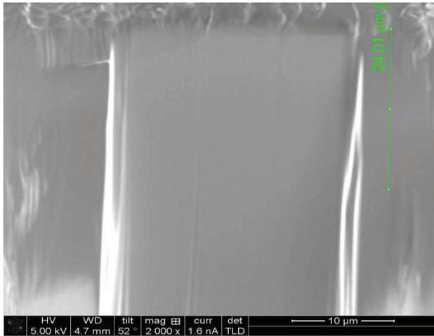
Figure 4: FIB image of sample #7 with a depth greater than 24 μm. Again, no nitride layer could be seen.
