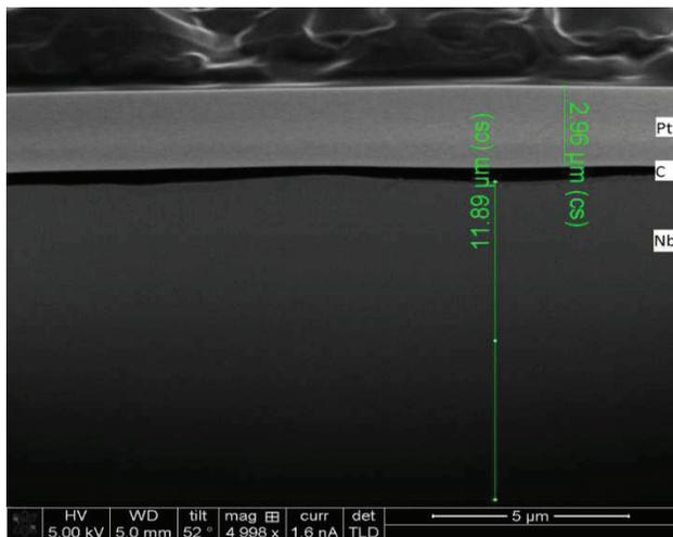
Figure 3: Focused Ion Beam Microscopy (FIB) image of the cross section of sample #7 (120 min Nitrogen exposure).
