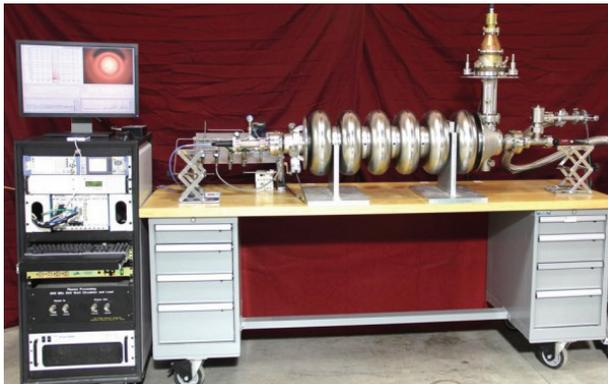
Figure 2: Plasma processing in a 6-cell beta=0.81 cavity at the SNS.
