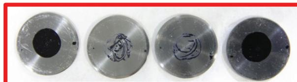
Figure 11: Nb samples after plasma processing in Ne-O<sub>2</sub>-H<sub>2</sub> mixture. The samples positioned near the end cells of the cavity were cleaned while the samples located near the end flanges remain basically unchanged.
