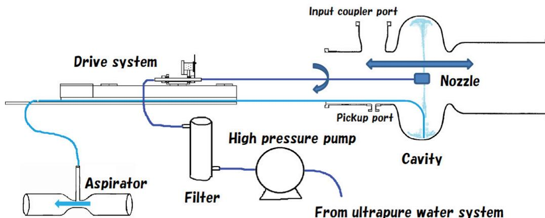
Figure 1: Schematic diagram of horizontal HPR apparatus.
