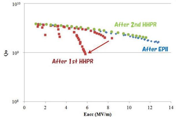
Figure 2: Q-Eacc curves of the prototype cavity after 1st and 2nd HHPR.
