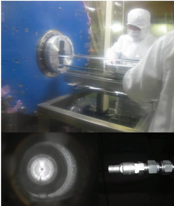
Figure 3: HHPR application to cavity module (top), and stainless steel nozzle and its water jets (bottom).
