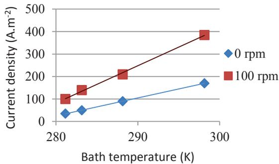
Figure 2: Limiting current (electropolishing current) as a function of bath temperature and mass transport.
