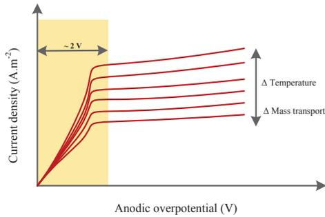
Figure 1: Schematic representation of trials made at different ( $\Delta$ ) temperatures and RDE speeds.
