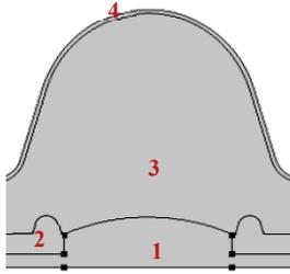
Figure 6: Final cathode geometry for SPL beta cell (radial axisymmetric cut): 1) cathode active surface; 2) insulated cathode surface; 3) electrolyte; 4) anode (SRF structure).
