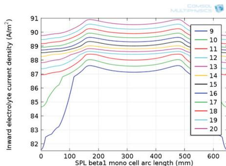
Figure 7: Current density distribution across SPL beta = 1 mono cell SRF structure. Each line corresponds to the applied potential in volts as shown in the legend.
