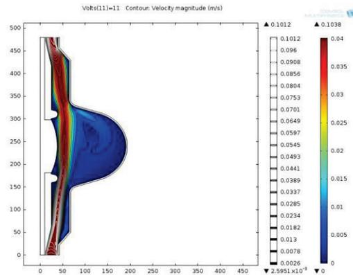
Figure 8: Bath speed distribution inside the SPL beta cell mono cell for a nominal flow of 1.2 m<sup>3</sup>/h. The scale is in m.s<sup>-1</sup>.
