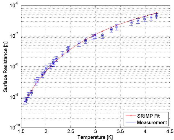
Figure 3: Fit of  $R_s$  vs Temperature using SRIMP to extract  $R_0$  and energy gap.
