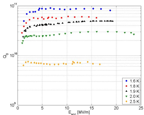
Figure 1:  $Q_0$  vs  $E_{acc}$  performance at 1.6, 1.8, 1.9, 2.0, 2.5 K. The error on  $Q_0$  is 20% and 10% on  $E_{acc}$ .
