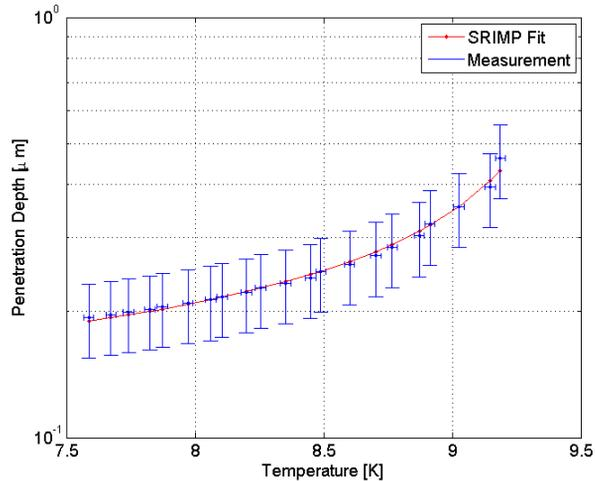
Figure 2: Fit of penetration depth vs Temperature using SRIMP to extract  $T_c$  and mean free path.
