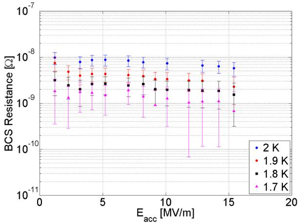
Figure 4: BCS Resistance vs  $E_{acc}$ .
