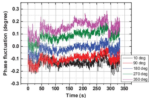
Figure 4: Phase stability of the prototype LLRF without feedback control
