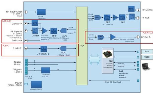
Figure 1: Block diagram of the prototype LLRF.
