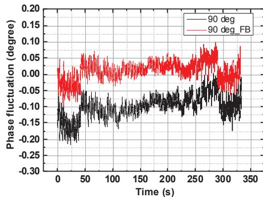
Figure 6: Phase stability of the prototype LLRF: compared with no feedback control and PID feedback control.
