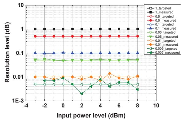
Figure 2: Power resolution of the prototype LLRF.
