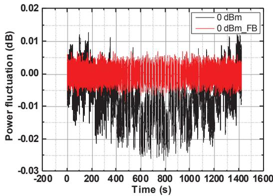
Figure 5: Amplitude stability of the prototype LLRF: compared with no feedback control and PID feedback control.
