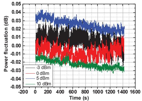
Figure 3: Amplitude stability of the prototype LLRF without feedback control.
