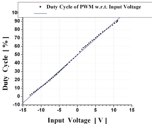
Fig. 6: Response of Pulse Width Modulator.
