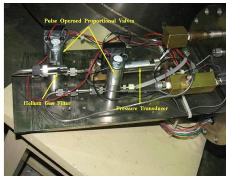
Fig. 4: Modified pneumatic frequency tuner.
