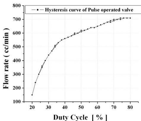
Fig. 7: Response of Valve in Pulse Mod.
