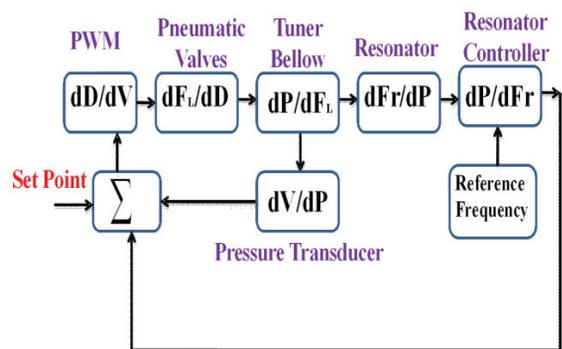
Fig. 5: Transfer Characteristics of modified pneumatic frequency tuner system.
