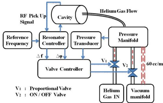
In the new system, dashed lines are not present and V1, V2 both are pulse operated Proportional Valves
