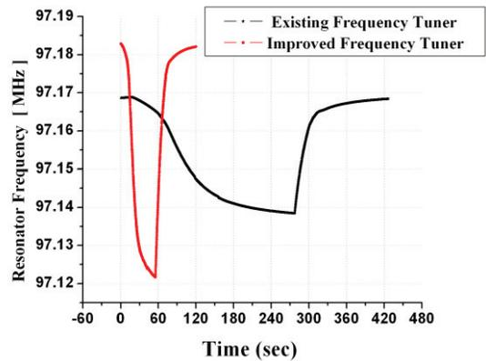
Fig. 8: Change of frequency of QWR by pressurizing and evacuating the tuner bellow.
