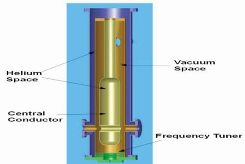
Fig. 2: The diagram of QWR with slow tuner bellow.
