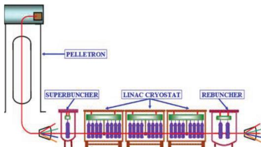
Fig. 1: Schematic diagram of Pelletron LINAC system.
