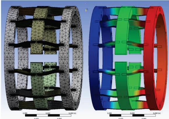
Figure 2: 3.9 GHz cavity tuner FE model developed for kinematics and stress analyses: mesh matrix (left), longitudinal strain distribution (right).
