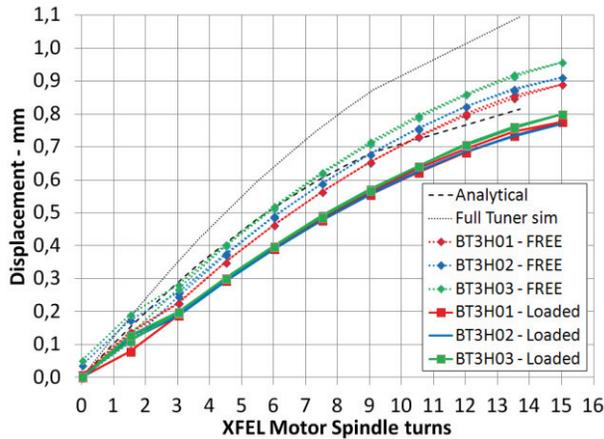
Figure 6: overview of room temperature tests on prototypes compared to simulations.
