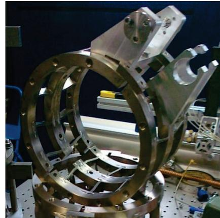
Figure 4: The 3.9 GHz cavity Blade Tuner.
