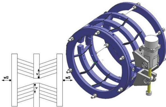
Figure 1: ILC Blade Tuner and its kinematics principle.
