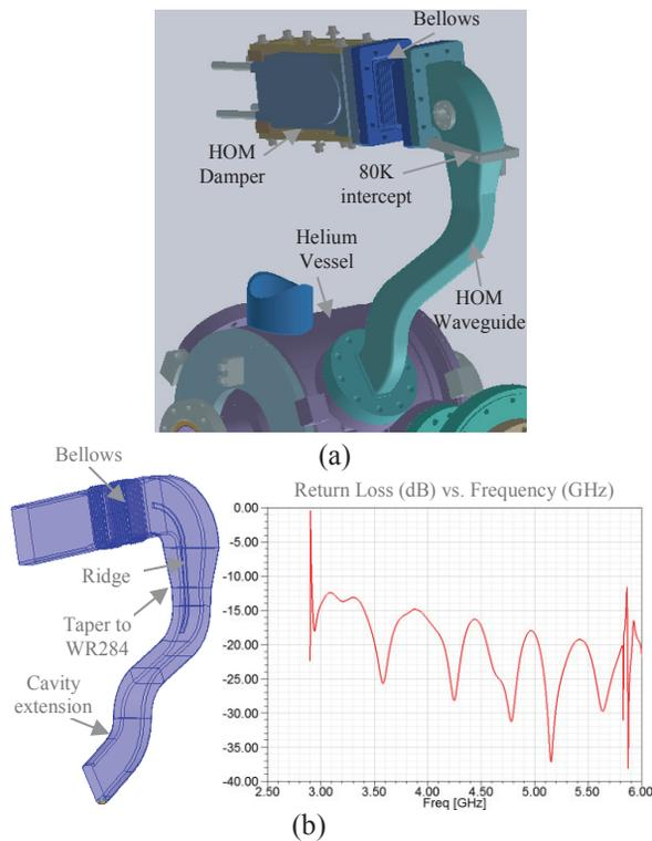
Figure 4: HOM waveguide assembly: (a) CAD geometry and (b) RF simulation model with return loss.
