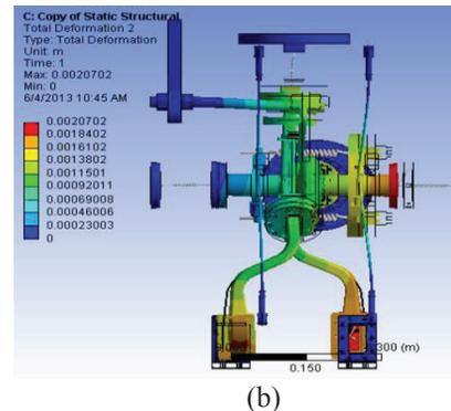
Figure 5: HOM waveguide thermal simulations: (a) heat load from static and dynamic effects with 5K and 80K thermal intercepts, and (b) displacement of cavity assembly due to temperature cycling to 2K. Bellows are represented as spring forces.
