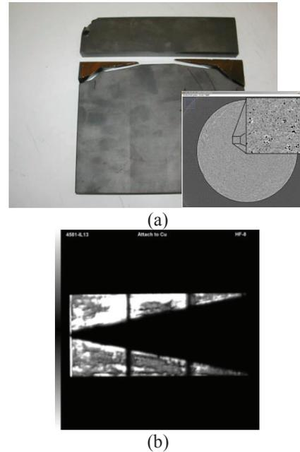
Figure 3: Manufacturing issues with HOM dampers: (a) St. Gobain iso-pressed SiC plate failure after single cut - inset shows a topography scan of SiC and (b) ultrasonic image of SiC tiles bonded to copper damper body. White areas denote regions where the solder is dis-bonded.
