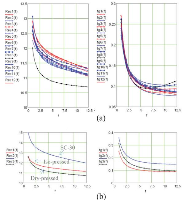
Figure 1: SiC electrical parameters: (a) permittivity and loss tangent for St. Gobain iso-pressed SiC, where the out-lying black line represents a sample with the largest dimensional deviation, and (b) averaged permittivity and loss tangent for St. Gobain iso-pressed, Coorstek SC-30, and St. Gobain dry-pressed SiC.
