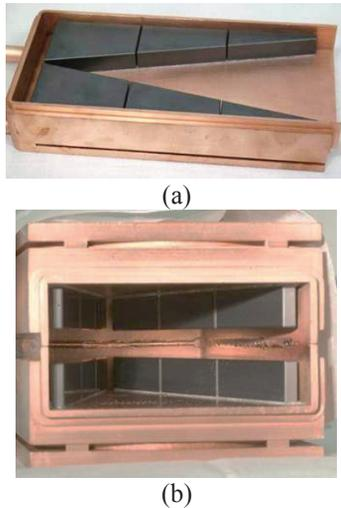
Figure 2: HOM damper assemblies: (a) copper damper half with soldered SiC tiles and (b) ebeam welded prototype damper assembly.
