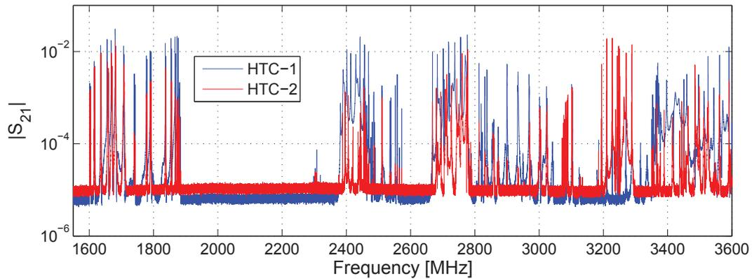
Figure 3: Amplitude of the scattering parameter  $S_{21}$  in the first two HTC experiments. The large quality factor of the modes are due to the fact that there were no HOM absorbing loads installed in HTC-1 and HTC-2. The mode frequencies agree with 2.5D simulations.
