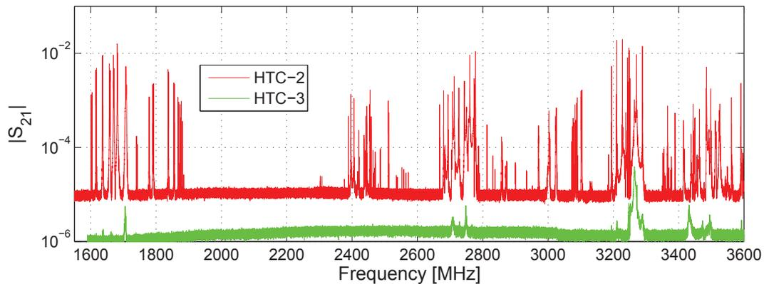
Figure 4: Amplitude of the scattering parameter  $S_{21}$  in the HTC-2 and HTC-3 experiments. The only significant change between the two runs is the addition of beamline absorbers in HTC-3. The measurements show a strong damping of all modes.
