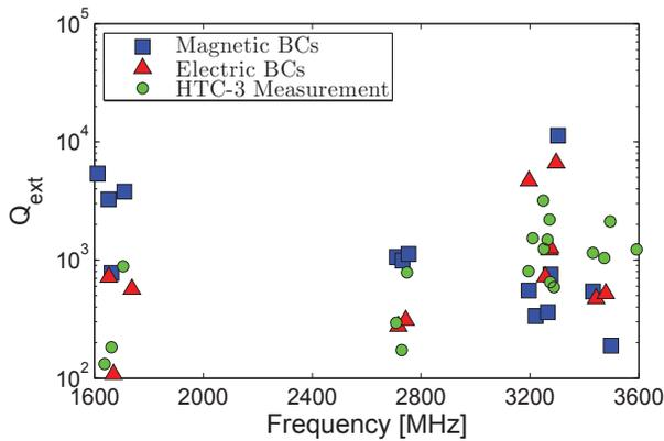
Figure 5: Comparison between HOMs measured in the HTC-3 and ACE3P simulations. Some discrepancy between the simulated and measured points is expected due to machining variation.
