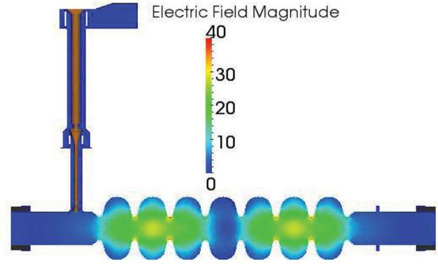
Figure 1: Magnitude of the electric field (in arbitrary units) for a dipole mode in the lowest HOM passband, ( $f=1612$ ,  $Q_L = 5.3 \times 10^3$ ). The absorbing load is in gray, and the white areas are alumina dielectrics isolating the cavity vacuum space from the cold and warm spaces.
