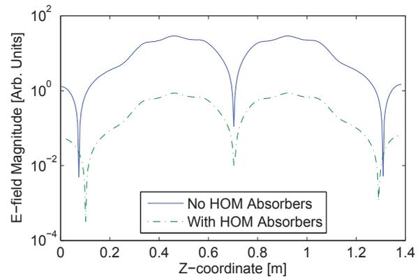
Figure 2: Magnitude of electric field along a line parallel to the beam axis and offset toward the high power coupler by 1 mm for a geometry with and without absorbing loads for the mode presented in Fig. 1. The absorbing load properties were  $\epsilon = (50 - 25i)\epsilon_0$  and  $\mu = \mu_0$ . Both cases have the same energy stored in the cavity, but energy is concentrated in the HOM load when it is present, reducing the field amplitude near the beam axis.
