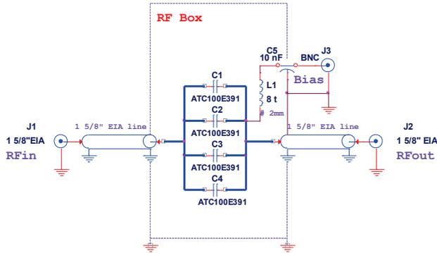
Figure 9: Electrical diagram of the 4 kW BIAS "T".
