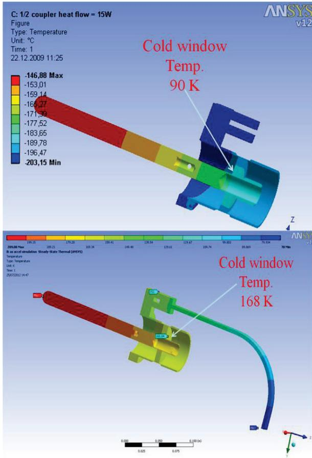
Figure 3: The cold window temperature maps without (top) and with (bottom) the copper braid, for 30 W generated uniformly on the coupler antenna.
