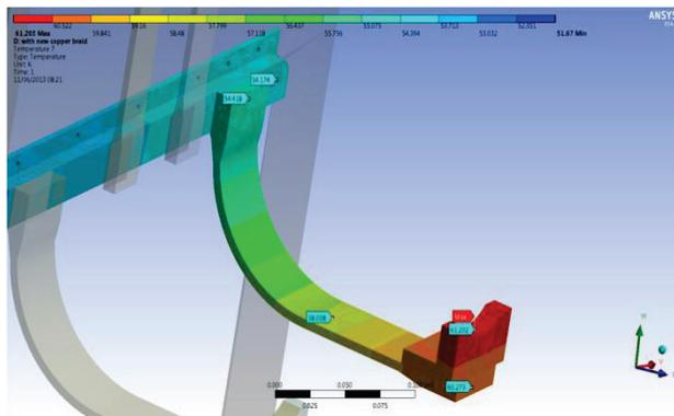
Figure 7: Temperature map of the cold window copper braid, including the IM contacts.
