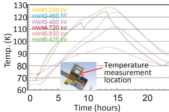
Figure 1: PSM HWRs couplers cold windows temperatures, measured during 0.2 mA beam operation.
