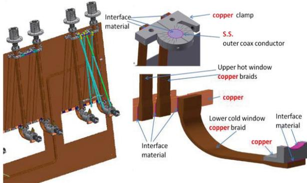
Figure 5: A layout of the copper braids heat leads and detailed views of the interface contacts.
