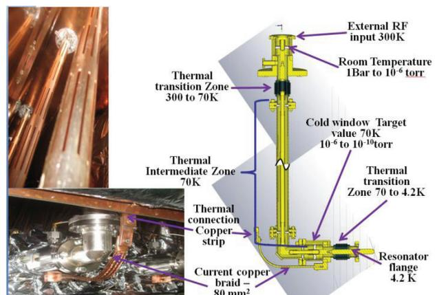
Figure 2: The SARAF PSM coupler thermal zones [2].
