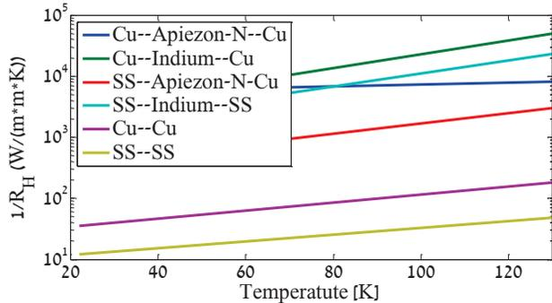
Figure 6: Heat conductance of the considered contacts as a function of temperature based on [6].
