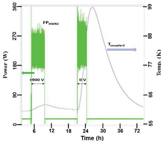
Figure 11: The cold window temperature rise time gradient with/without a 900 V bias voltage.
