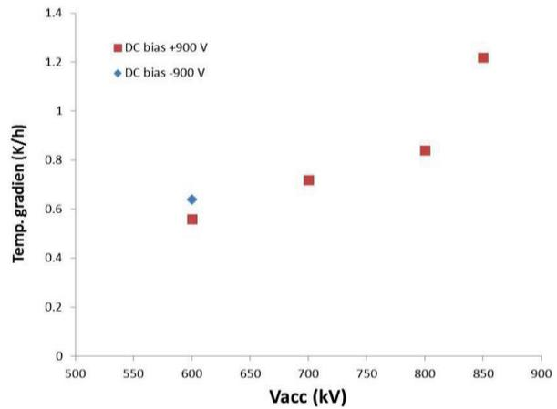
Figure 12: The temperature rise gradient as a function of the cavity voltage.
