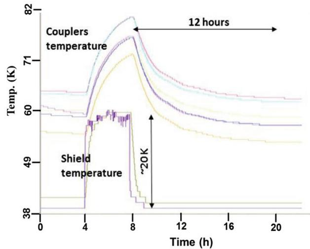
Figure 8: Cold window temperature as a function of time following 20 K upward and downward step changes in the thermal shield He gas loop.
