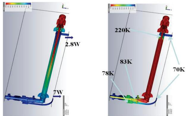
Figure 4: Configuration C. Left: Heat loads. Right: Temperatures.
