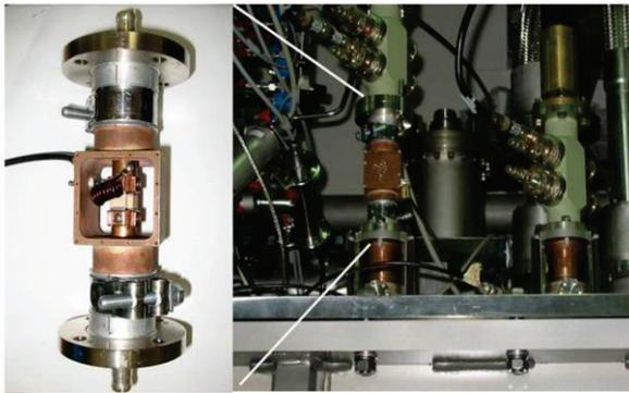
Figure 10: Left: the bias T prototype, Right: As installed on the ambient coupler window at the PSM top lead.
