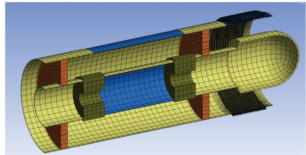
Figure 2: RF power coupler design after the optimization.
