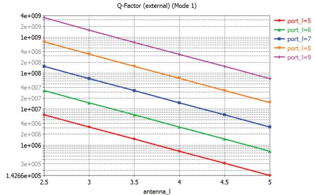
Figure 5: External Q-factor as function of the antenna's length for different RF port dimensions.
