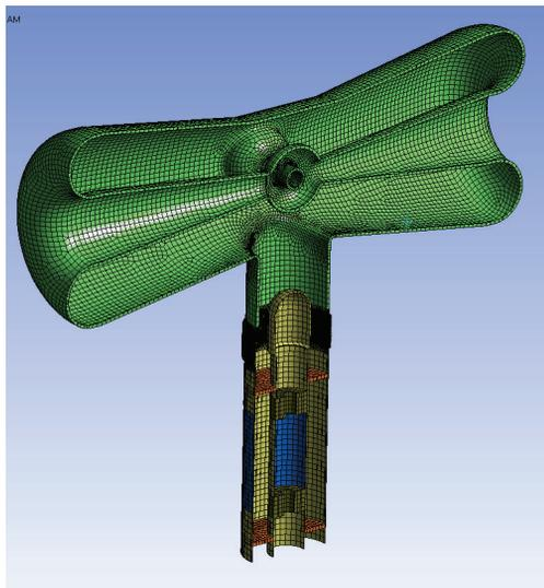
Figure 4: Power coupler connected to the HWR.
