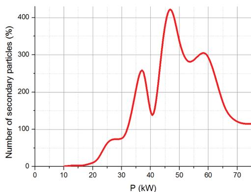
Figure 7: Relative counter function for RF coupler.
