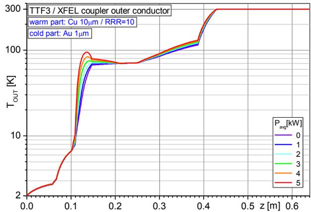
Figure 12:  $T_{out}(z)$  with 1 $\mu\text{m}$  gold on cold outer conductor.
