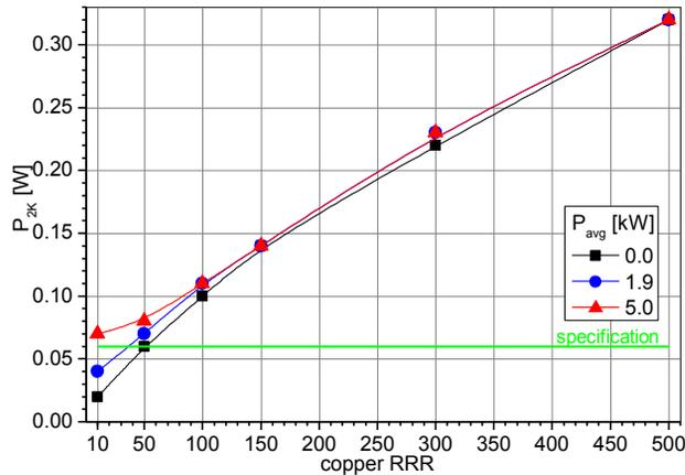
Figure 5: 2.0 K heat load with copper RRR.
