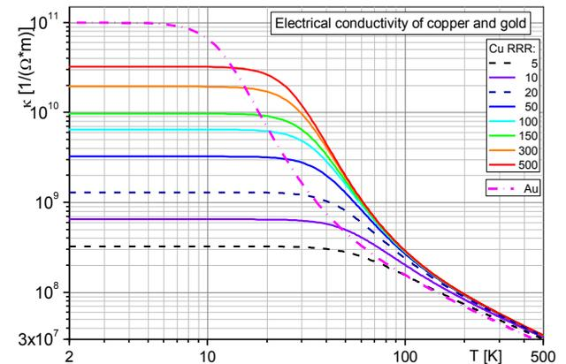
Figure 3: Electrical conductivity of copper and gold.
