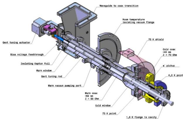
Figure 1: XFEL RF power input coupler.
