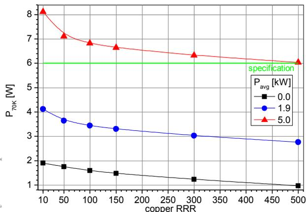
Figure 7: 70 K heat load with copper RRR.
