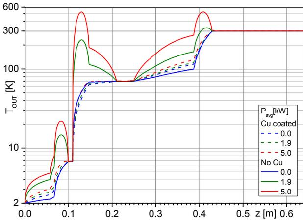
Figure 10: Outer conductor  $T(z)$  without copper layer.
