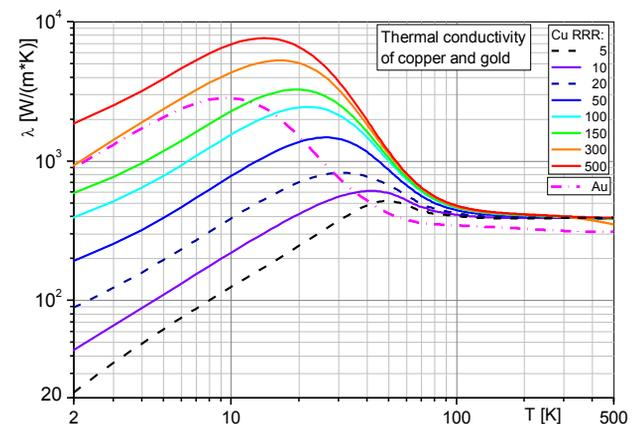
Figure 4: Thermal conductivity of copper and gold.
