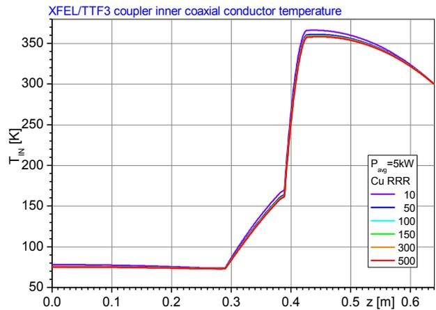
Figure 8: Inner conductor T(z) with copper RRR.
