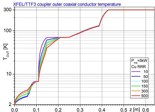
Figure 9: Outer conductor T(z) with copper RRR.
