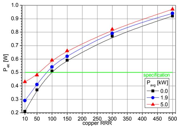
Figure 6: 4.2 K heat load with copper RRR.
