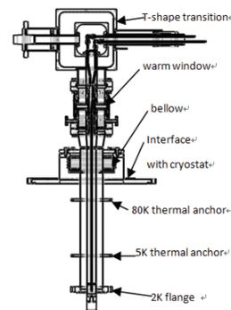
Figure 1: Cross section of the input coupler
