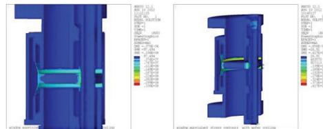
Figure 4: Thermal stress on the ceramic window (left: without cooling; right: with water cooling)
