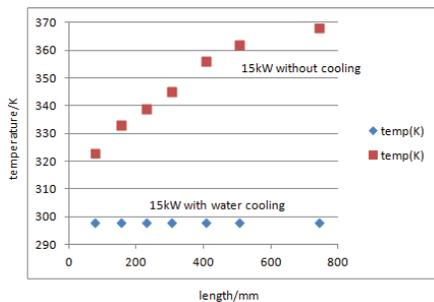
Figure 2: Temperature distributions along inner conductor
