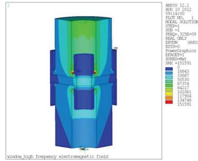
Figure 3: Distribution of electric field at 15kW, TW
