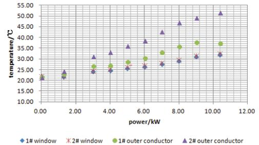
Figure 9: Temperature as a function of RF heating
