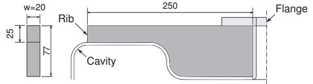
Figure 5: A rib on an end-wall of the cavity.
