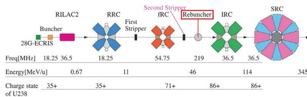
Figure 1: Accelerating mode for very heavy ions ( $^{238}\text{U}$  beam).
