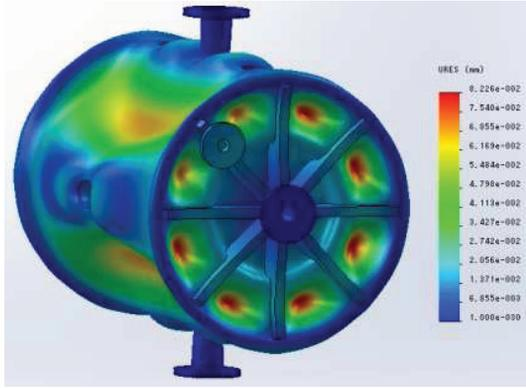
Figure 7: Deformation of Nb cavity with fixed beam ports.
