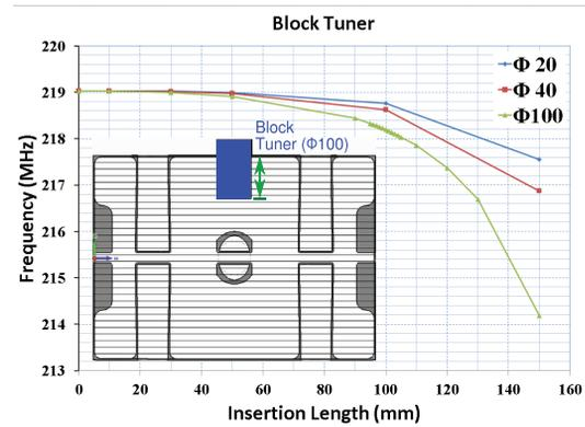
Figure 4: Frequency tuning by a block tuner.
