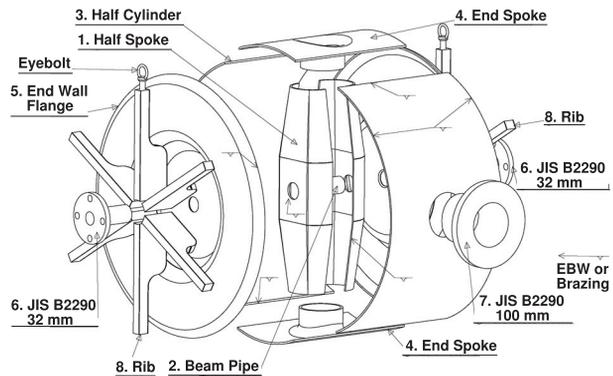
Figure 10: Parts for single-spoke model.
