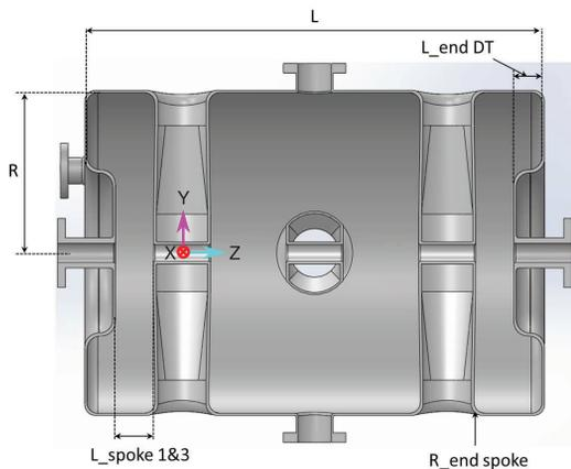
Figure 8: Geometrical parameters considered for manufacturing errors.
