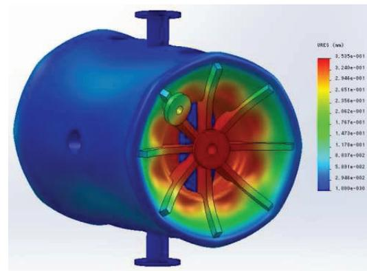
Figure 6: Deformation of Nb cavity with unfixed beam ports.
