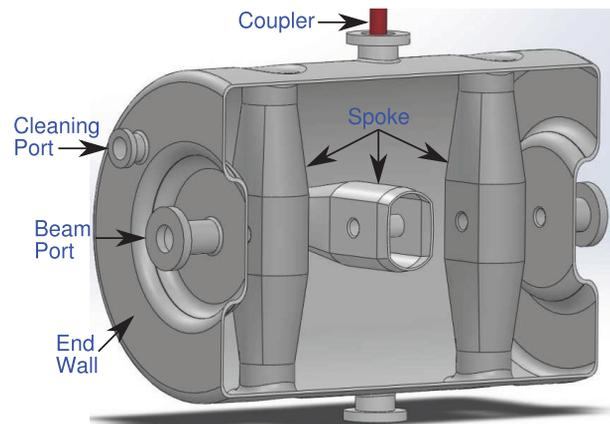
Figure 2: Triple-spoke cavity.
