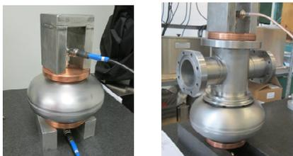
Figure 6: RF jig for ‘smart-bell’ frequency measurement
